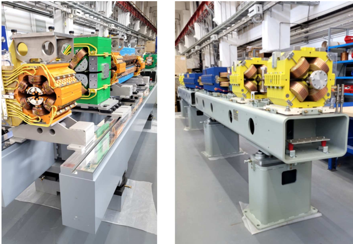
Figure 6. Magnet assemblies on girders for the storage ring (left) and for SKIF synchrotron [9].
