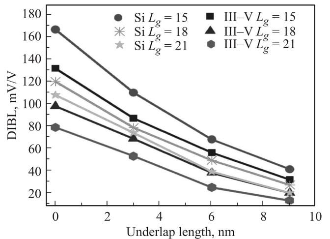
**Figure 3.** Dependence of DIBL on underlap length  $L_{un}$ , for both devices. The gate length  $L_g$  is varied from 15 to 21 nm in steps of 3 nm. The underlap length  $L_{un}$  is varied from 0 to 9 nm in steps of 3 nm.  $DIBL = [(V_{th1} - V_{th2}) / (V_{ds1} - V_{ds2})]$  where  $V_{th1}$  and  $V_{th2}$  are threshold voltages extracted at drain bias of  $V_{ds1} = 50$  mV and  $V_{ds2} = 1.0$  V.
