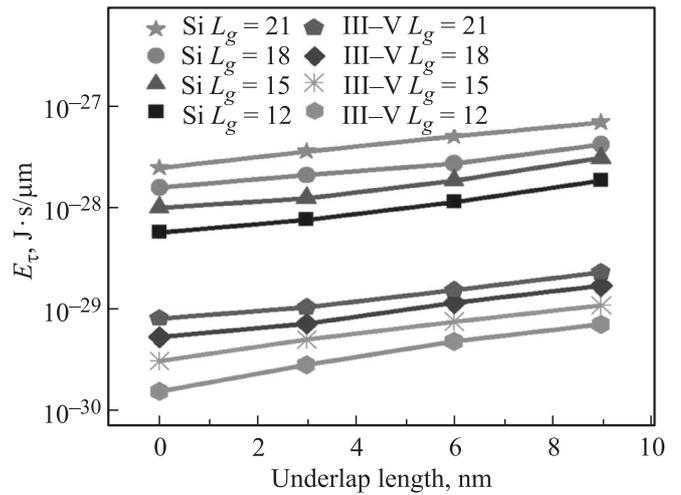
**Figure 7.** Energy delay product versus underlap length  $L_{un}$ , for both devices. The gate length  $L_g$  is varied from 12 to 21 nm in steps of 3 nm. The underlap length  $L_{un}$  is varied from 0 to 9 nm in steps of 3 nm. Energy delay product  $E_t = (CV/I) \cdot (CV^2)$ .
