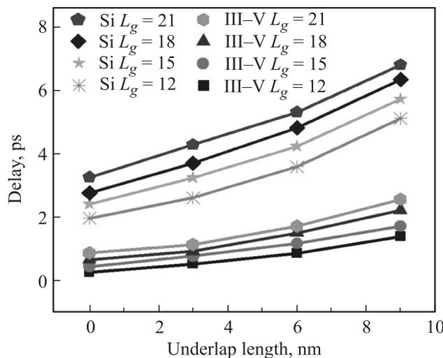
**Figure 6.** Intrinsic delay variation with underlap length  $L_{un}$ , for both devices. The gate length  $L_g$  is varied from 12 to 21 nm in steps of 3 nm. The underlap length  $L_{un}$  is varied from 0 to 9 nm in steps of 3 nm. Delay =  $CV/I$ .
