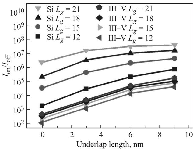
**Figure 5.**  $I_{on}/I_{off}$  ratio variation with underlap length  $L_{un}$ , for both devices. The gate length  $L_g$  is varied from 12 to 21 nm in steps of 3 nm. The underlap length  $L_{un}$  is varied from 0 to 9 nm in steps of 3 nm.
