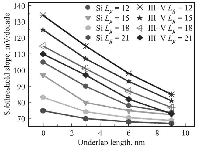
**Figure 4.** Subthreshold slope versus underlap length  $L_{un}$ , for both devices. The gate length  $L_g$  is varied from 12 to 21 nm in steps of 3 nm. The underlap length  $L_{un}$  is varied from 0 to 9 nm in steps of 3 nm.  $SS = \Delta V_g / \Delta(\lg I_D)$ .
