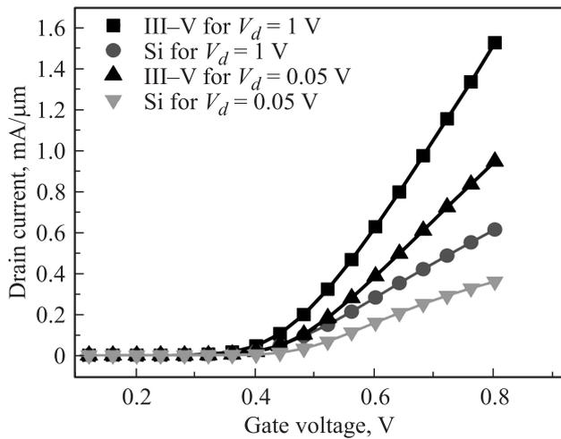
**Figure 2.**  $I_D$  versus  $V_g$  characteristics of both devices, with constant gate length  $L_g = 18$  nm, body thickness  $t_b = 6$  nm and underlap length  $L_{un} = 5$  nm. The applied drain voltage is  $V_d = 0.05$  V and  $V_d = 1$  V for both devices.
