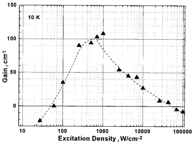
**Figure 4.** Gain vs excitation density in the structure with excitonic waveguide.
