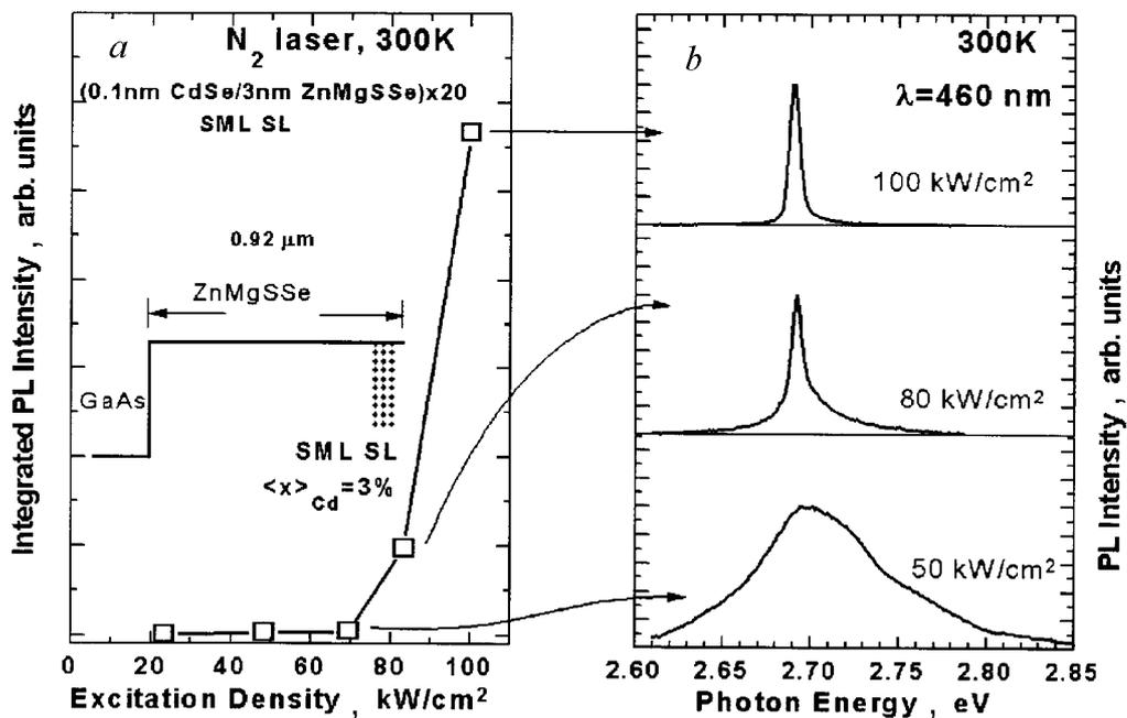
**Figure 3.** Dependence of integrated PL intensity versus excitation density (a) and luminescence spectra (b) of the excitonic waveguide structure.
