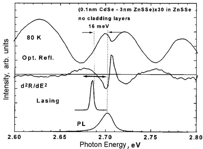
**Figure 2.** Photoluminescence, lasing, and optical reflectance spectra of the excitonic waveguide structure.
