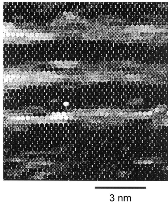
**Figure 1.** Local lattice parameter image of the structure with CdSe insertions in a ZnSe matrix.
