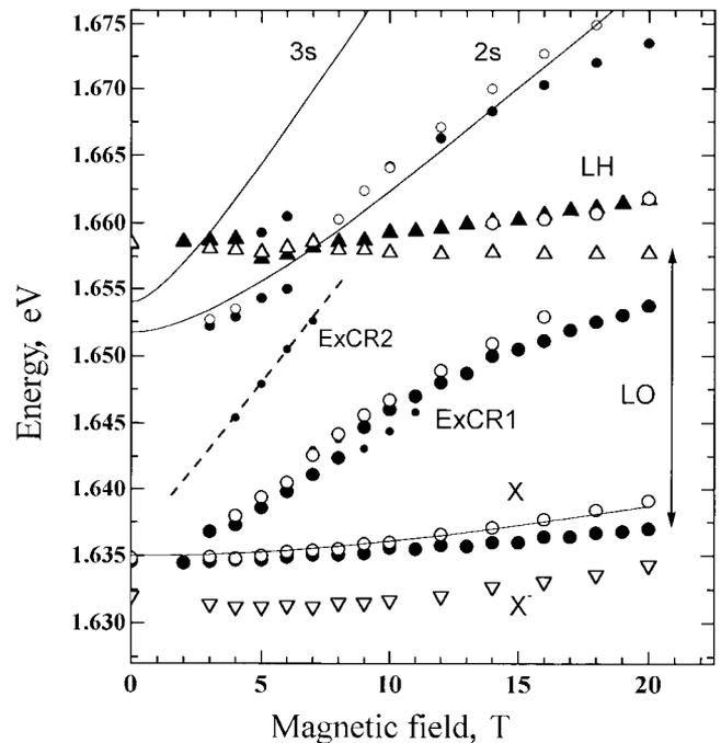
**Figure 6.** Fan chart of an 8 nm CdTe/Cd<sub>0.7</sub>Mg<sub>0.3</sub>Te quantum well. Open symbols represent  $\sigma^+$  and closed symbols  $\sigma^-$  polarization respectively. The lines represent calculation for the exciton 1s, 2s and 3s state applying the model described in ref. [18].
