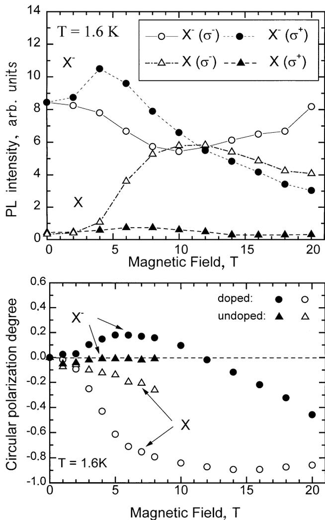
**Figure 3.** Magnetic field variation of the PL line intensities detected for different circular polarizations for an 8 nm-thick CdTe/Cd<sub>0.7</sub>Mg<sub>0.3</sub>Te modulation-doped QW (upper panel). Magnetic-field-induced circular polarization degree of the exciton and negatively charged exciton PL lines with (circles) and without (triangles) modulation doping (lower panel).
