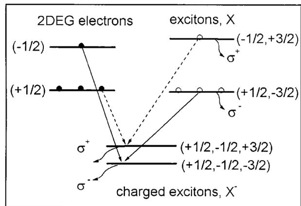
**Figure 2.** Schematical presentation of an *X*<sup>−</sup> formation process in external magnetic fields from excitons and 2DEG electrons.
