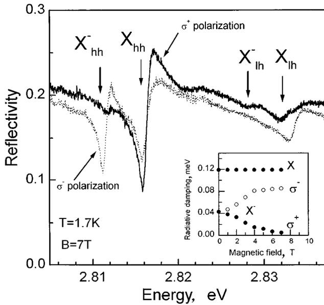
**Figure 5.** Reflectivity spectra of a 10 nm ZnSe/Zn<sub>0.89</sub>Mg<sub>0.11</sub>S<sub>0.18</sub>Se<sub>0.82</sub> quantum well at 1.6 K and 7 T for  $\sigma^+$  (solid) and  $\sigma^-$  (dashed) lines. The insert shows the radiative damping (oscillator strength) for the exciton and the trion.
