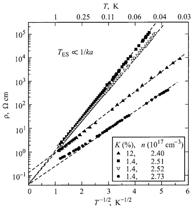
**Figure 1.** Temperature dependence of resistivity at low compensation,  $K = 0.014, 0.12$ .
