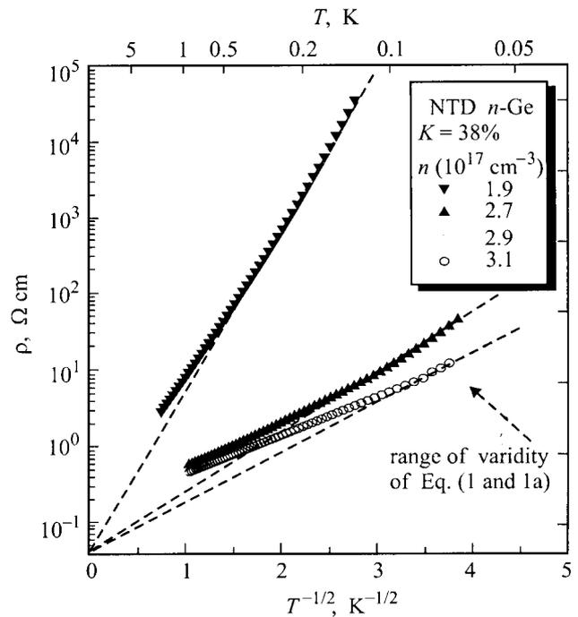
**Figure 2.** Temperature dependence of resistivity at medium compensation,  $K = 0.38$ .
