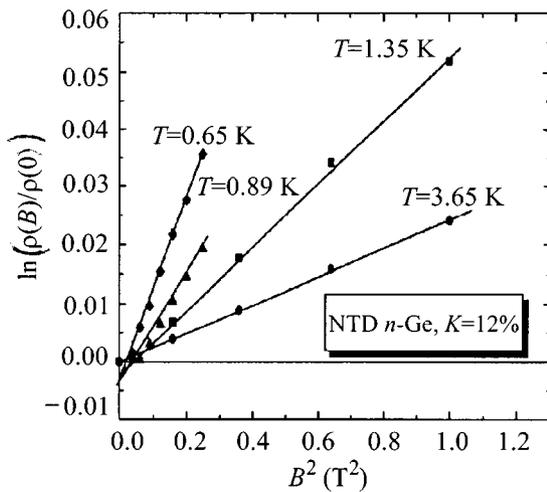
Figure 5. Typical dependence of the hopping magnetoresistance of  $B^2$ .
