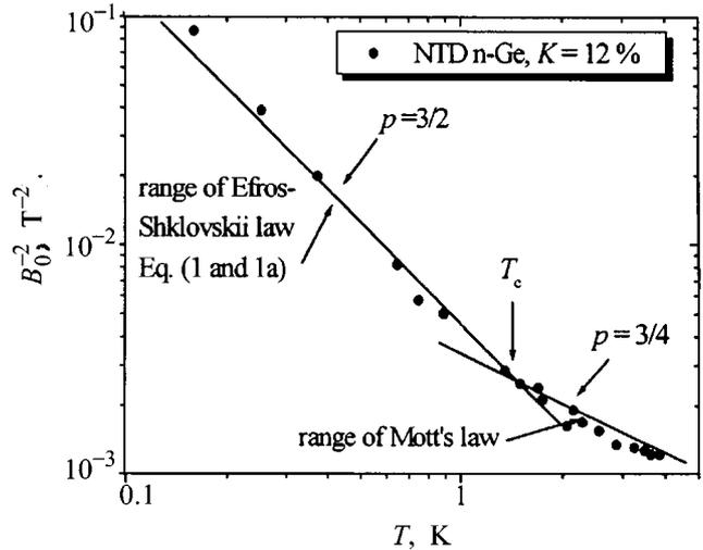
Figure 6. Temperature dependence of the positive hopping magnetoresistance. The upper straight line shows the range of validity of Eq. (4).
