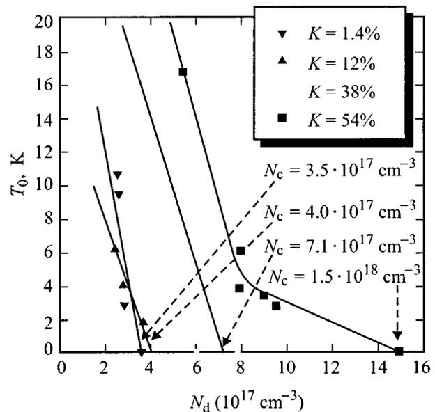
**Figure 3.** Determination of  $N_c$  at  $T_0 \rightarrow 0$ .
