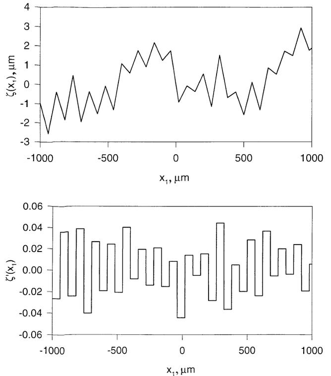
**Figure 2.** Numerical generation of a surface profile and its derivative. The parameters employed are  $b = 60 \mu\text{m}$ ,  $m = 1$ ,  $\gamma_m = 1$  and  $\theta_m = 5^\circ$ .
