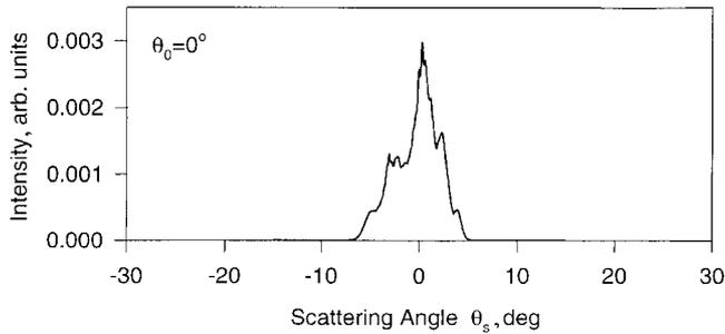
**Figure 9.** Experimental result for the angular dependence of the intensity of  $s$ -polarized light of wavelength  $\lambda = 0.6328 \mu\text{m}$  transmitted through a photoresist film. The angle of incidence is  $\theta_0 = 0^\circ$ . The illuminated surface of the film is a one-dimensional random surface through which light is transmitted within the angle  $-5^\circ < \theta_s < 5^\circ$ , and is not transmitted outside this range.
