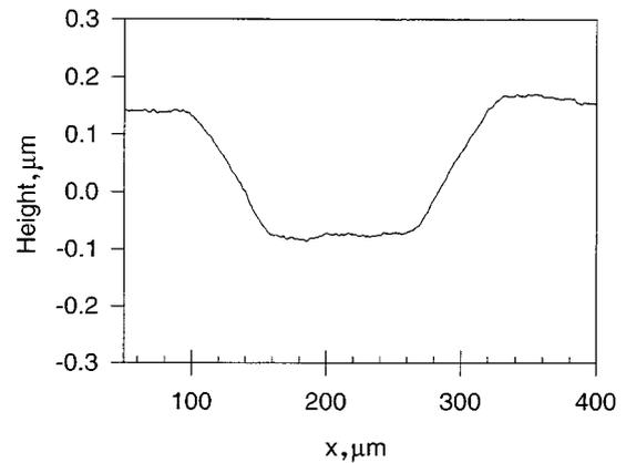
Figure 7. Measured profile that illustrates the experimental realization of the function  $s(x_1)$ . The profile was measured by means of a Dektak<sup>(st)</sup> mechanical profilometer.
