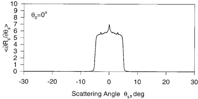
**Figure 3.** The mean differential reflection coefficient for normal incidence calculated from  $N_p = 3000$  realizations of the surface profile function. The parameters employed are  $\lambda = 0.6328 \mu\text{m}$ ,  $b = 60 \mu\text{m}$ ,  $m = 1$ ,  $\gamma_m = 1$ , and  $\theta_m = 5^\circ$ . The sampling interval on the surface was  $\Delta x = b/N = 0.2 \mu\text{m}$  ( $N = 300$ ), and the length of the surface was  $L_1 = 2000 \mu\text{m}$ .
