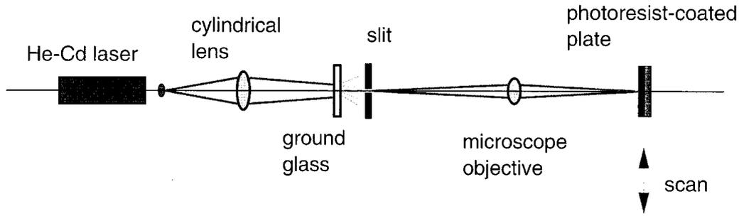
Figure 6. Schematic diagram of the experimental arrangement employed for the fabrication of the diffusers.
