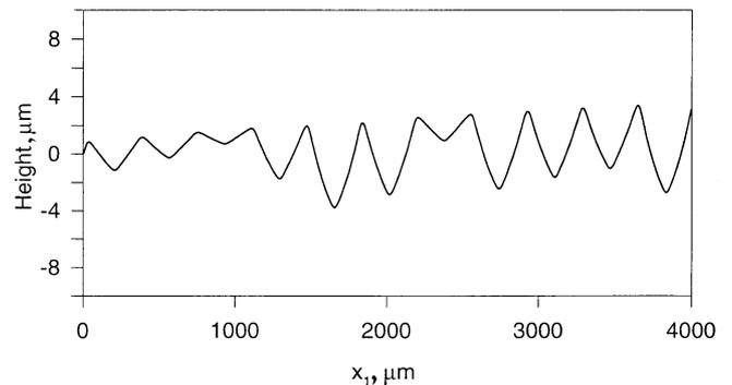
Figure 8. Measured segment of a surface profile for a fabricated sample. The parameters are  $b = 60 \mu\text{m}$ ,  $m = 0$ .
