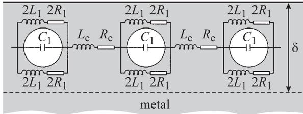
Figure 1. Nanoporous surface of metal and its equivalent circuit.
