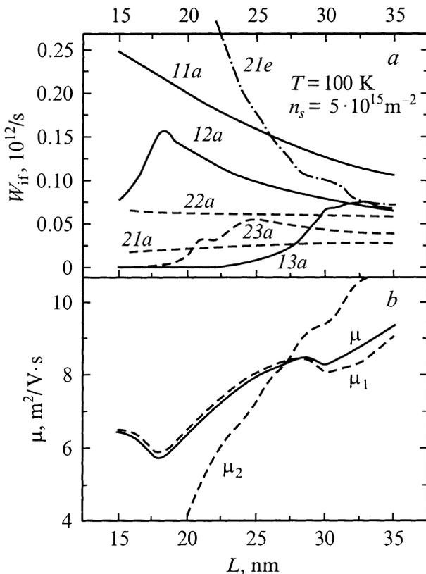
**Figure 2.** The electron-PO-phonon scattering rates  $W_{if}$  (*a*) and the subband and total electron mobilities (*b*) as functions of QW width at  $n_s = 5 \cdot 10^{15} \text{ m}^{-2}$ . Notations are as in Fig. 1.
