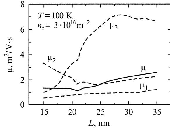
**Figure 3.** The subband and total electron mobilities as functions of QW width at  $n_s = 3 \cdot 10^{16} \text{ m}^{-2}$ . Notations are as in Fig. 1.
