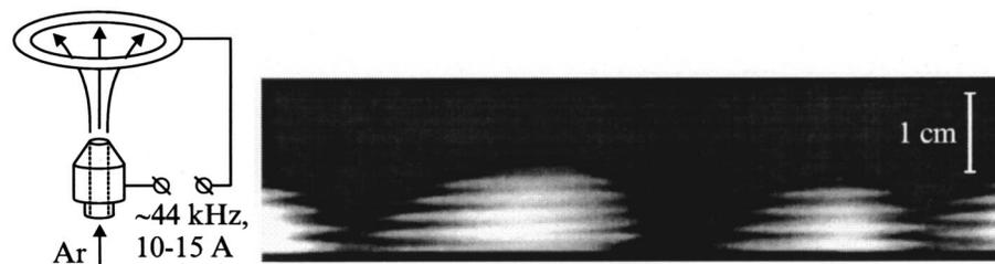
**Figure 2.** The principal scheme of the discharge in an argon flow at atmospheric pressure and a photo-registration of the irradiation intensity of the plasma discharge revealing forced running ionization waves. The current of the discharge arc is 7 A, the frequency is 44 kHz, and the linear rate of argon flow is 42 m/s. The hole of the central electrode is about 2.0 mm in diameter.
