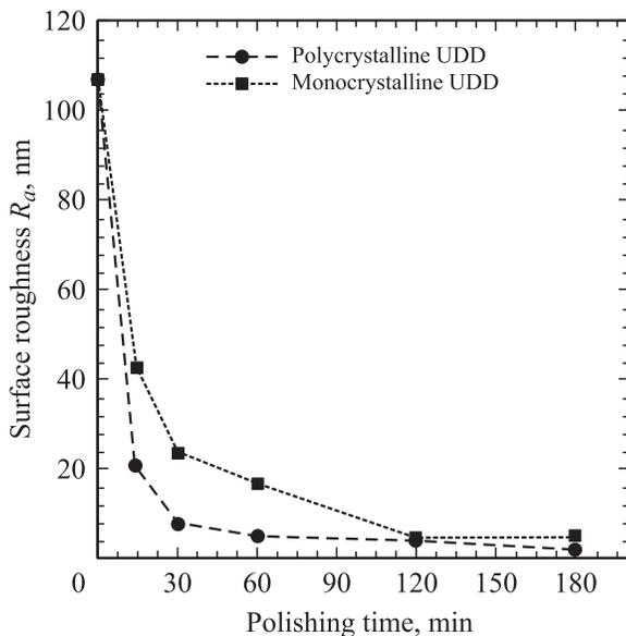
**Figure 4.** Surface roughness obtained using foamed polyurethane pad.
