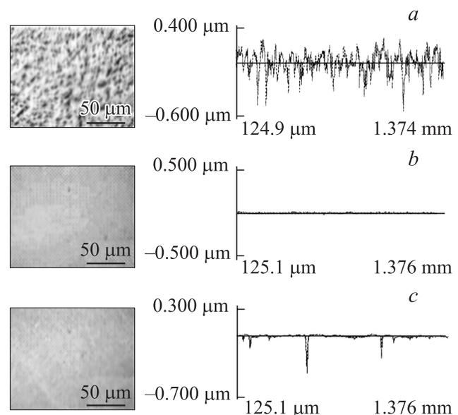
**Figure 5.** Optical micrographs of surfaces polished by new polishing pad with self-generating porosity. *a* — prior to polishing,  $R_a = 107$  nm; *b* — polycrystalline UDD,  $t = 90$  min,  $R_a = 2$  nm; *c* — monocrystalline UDD,  $t = 90$  min,  $R_a = 12$  nm.
