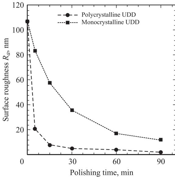
**Figure 3.** Surface roughness obtained using new polishing pad with self-generating porosity.
