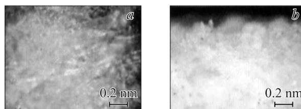
**Figure 2.** Optical micrographs of new pad with self-generating porosity. *a* — surface, *b* — cross-section.
