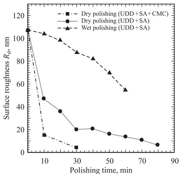
**Figure 1.** Results of polishing tests using ultra-fine grinding wheels.
