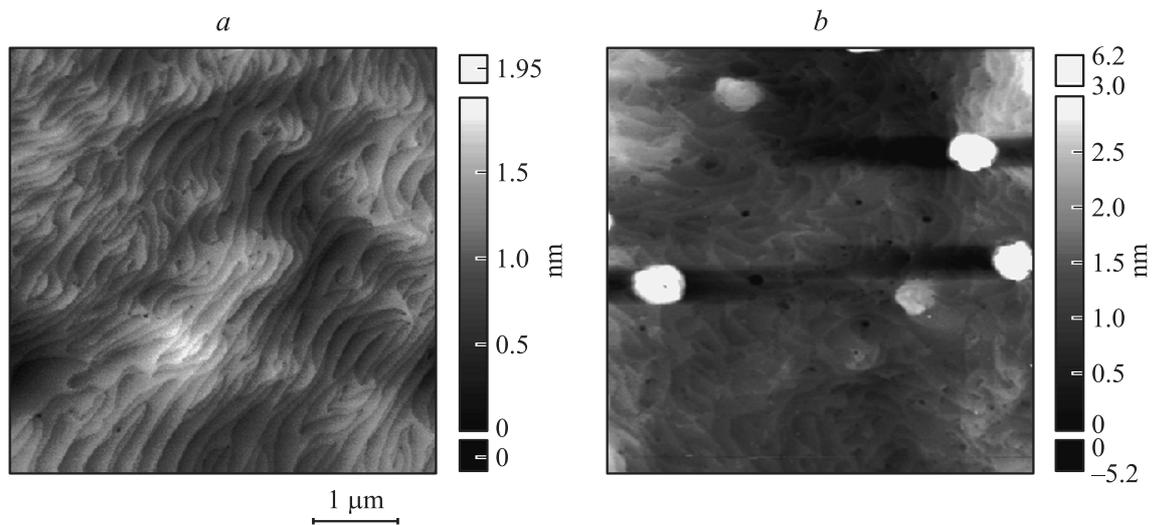
**Figure 1.** AFM scans with a  $5 \times 5 \mu\text{m}^2$  area of the samples: (a) A and (b) B. Dark to white color variance corresponds to pit to hill variance on the surface of the samples.
