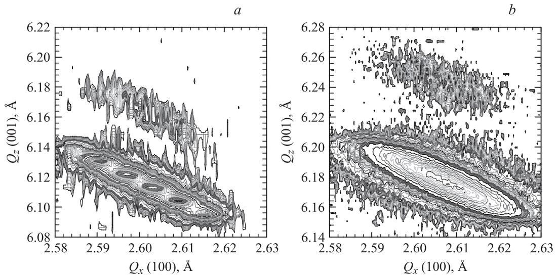
**Figure 3.** RSMs recorded around the asymmetric  $(10\bar{1}5)$  reflections for samples (a) A and (b) B.
