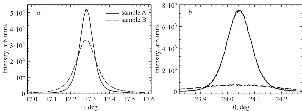
**Figure 2.** Bragg reflections of the samples: *a* — symmetric GaN (0002), *b* — asymmetric GaN (10 $\bar{1}2$ ).
