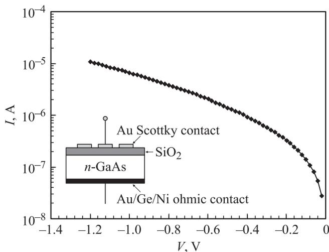
Figure 2. Reverse-bias semilogarithmic current–voltage characteristics of Au/SiO<sub>2</sub>/n-GaAs SCs at 300 K (inset figure shows structure of the SCs).
