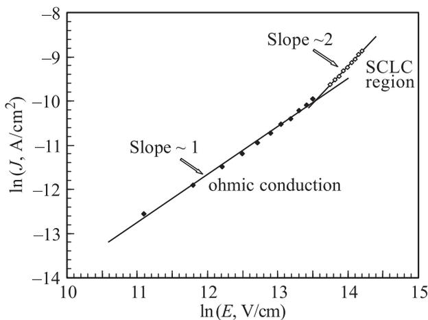
**Figure 5.**  $\ln(J)$  vs.  $\ln(E)$  plot at negative bias for Au/SiO<sub>2</sub>/n-GaAs SCs.
