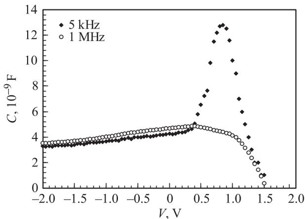
**Figure 4.**  $C$ - $V$  plots of low (5 kHz) and high (1 MHz) frequencies for Au/SiO<sub>2</sub>/n-GaAs SCs.
