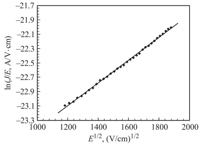
Figure 3. A plot of  $\ln(J/E)$  vs.  $\sqrt{E}$  at negative bias for Au/SiO<sub>2</sub>/n-GaAs SCs.
