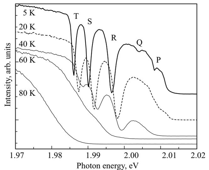
**Figure 3.**  $\text{BiI}_3$  absorption spectra in the temperature interval of 5–45 K. R, S and T lines are the stacking fault excitons (SFE), P and Q lines are excitons bound on fine impurities.
