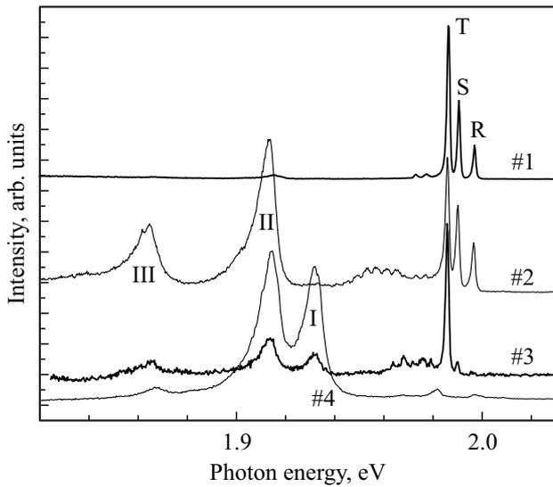
**Figure 1.** Luminescence spectra of  $\text{BiI}_3$  (samples 1–4) at  $T = 5$  K. Lines R, S, T refer to stacking fault excitons (SFE), stripes I, II, III refer to excitons of domains with the  $D_{3d}$  symmetry.
