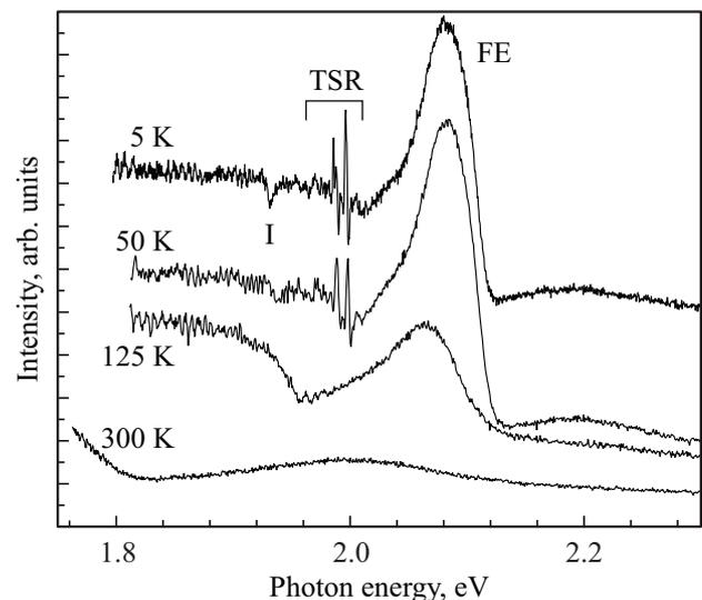
**Figure 4.** Evolution of the  $\text{BiI}_3$  crystal spectrum obtained in the reflection geometry in the temperature interval of 5–300 K.
