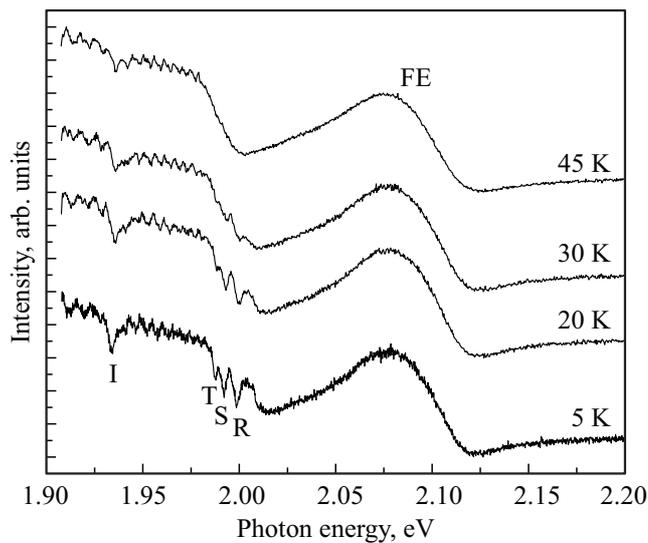
**Figure 2.**  $\text{BiI}_3$  spectra obtained in the reflection geometry in the temperature interval of 5–40 K. FE is the contour of free exciton stripe.
