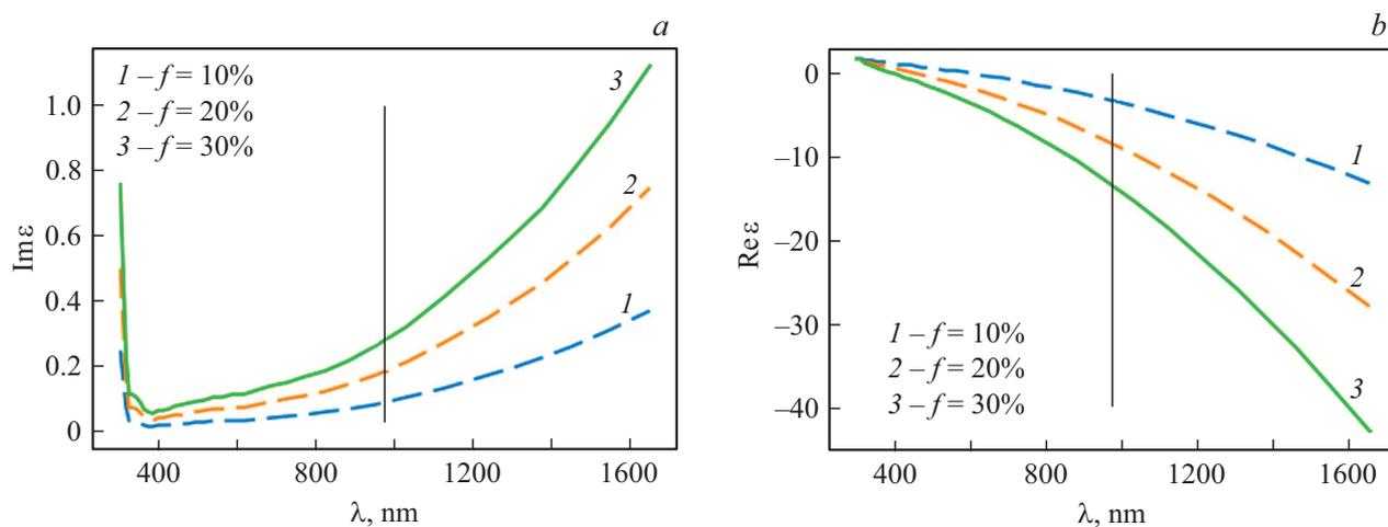
**Figure 1.** Spectra of imaginary (a) and real (b) parts of the effective permittivity of the hybrid material with different volume fractions of silver nanoparticles. The vertical line marks the operating frequency of semiconductor lasers based on GaAs (980 nm).
