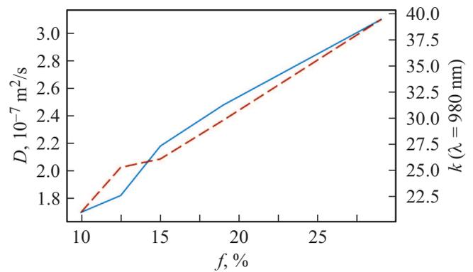
**Figure 3.** Dependences of effective temperature conductivity  $D$  (solid curve) and imaginary part  $k$  of the refraction coefficient at a wavelength of 980 nm (dashed curve) on the volume fraction of silver nanoparticles.
