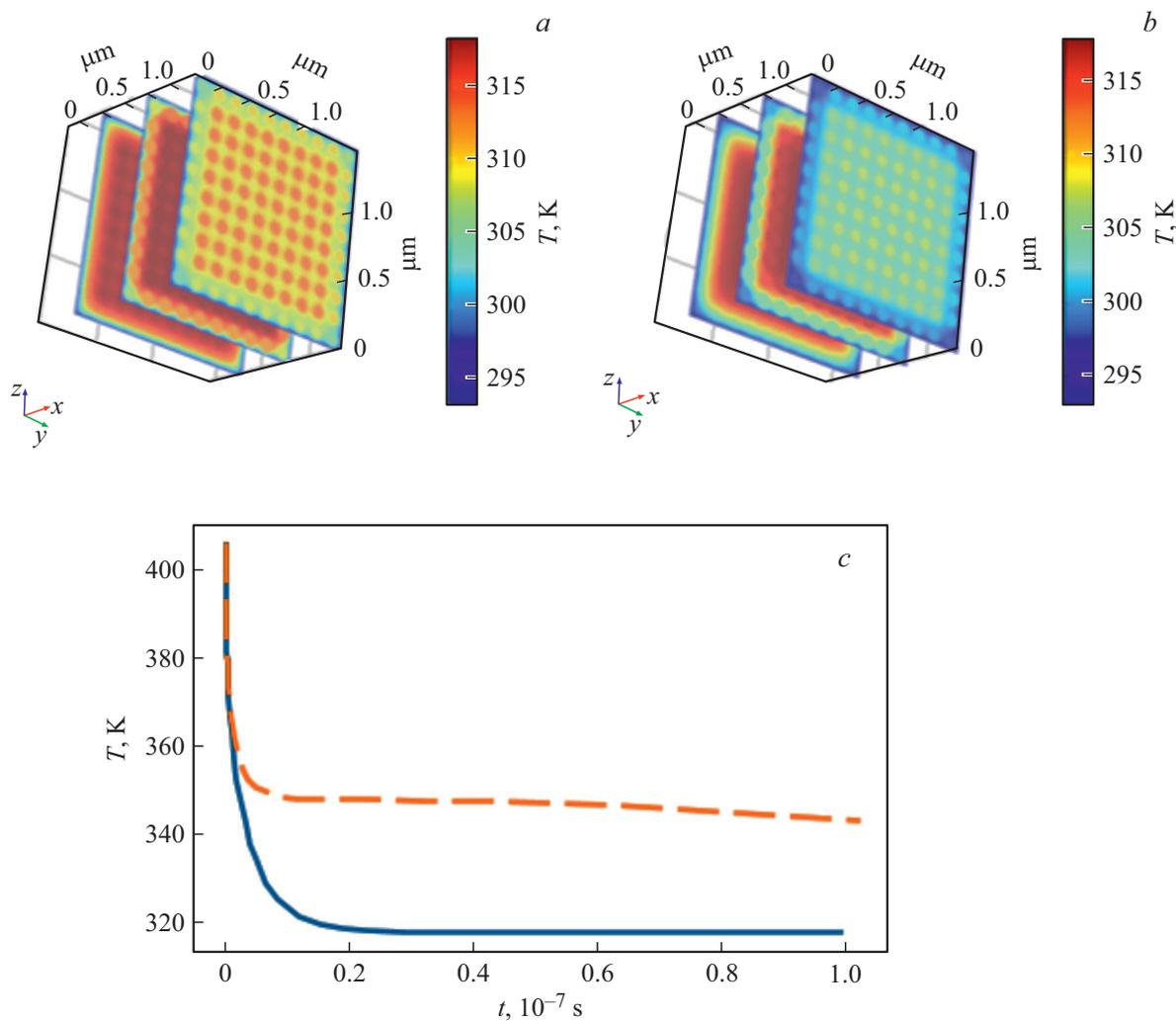
**Figure 2.** Temperature distribution in the structure with a volume fraction of nanoparticles of 29% within 40 (a) and 60 ns (b). c — temperature reduction with time in the process of cooling of materials with a volume fraction of particles of 17% (solid curve) and 29% (dashed curve).
