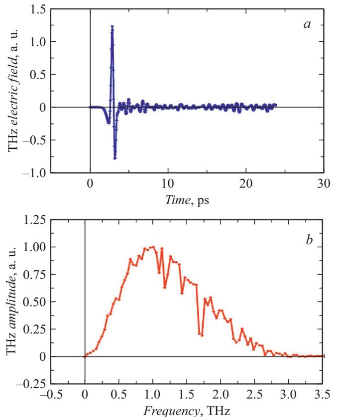
**Figure 2.** THz radiation generated in an epitaxial InAs layer on a heavily doped GaAs substrate. *a* — waveform of a THz pulse normalized by  $E(SI)_{\max}$ ; *b* — normalized THz radiation spectrum.
