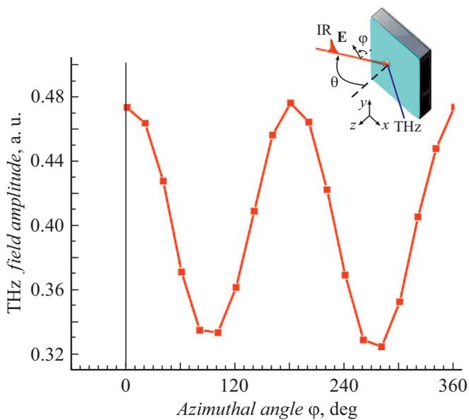
**Figure 3.** Polarization dependence of the THz field. The geometry of the experiment is shown in the inset ( $\theta$  is the incidence angle).
