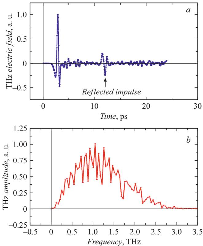
**Figure 1.** THz radiation generated in an epitaxial InAs layer on a semi-insulating GaAs substrate. *a* — waveform of a THz pulse normalized by  $E(SI)_{\max}$ ; *b* — normalized THz radiation spectrum.  $E(SI)_{\max}$  is the maximum amplitude of the electric field of THz radiation generated in an epitaxial InAs layer on a semi-insulating GaAs substrate.
