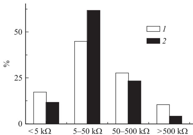
**Figure 3.** Resistance values distribution for ensembles of initial MWCNTs (1) and plasma treated MWCNTs (2).
