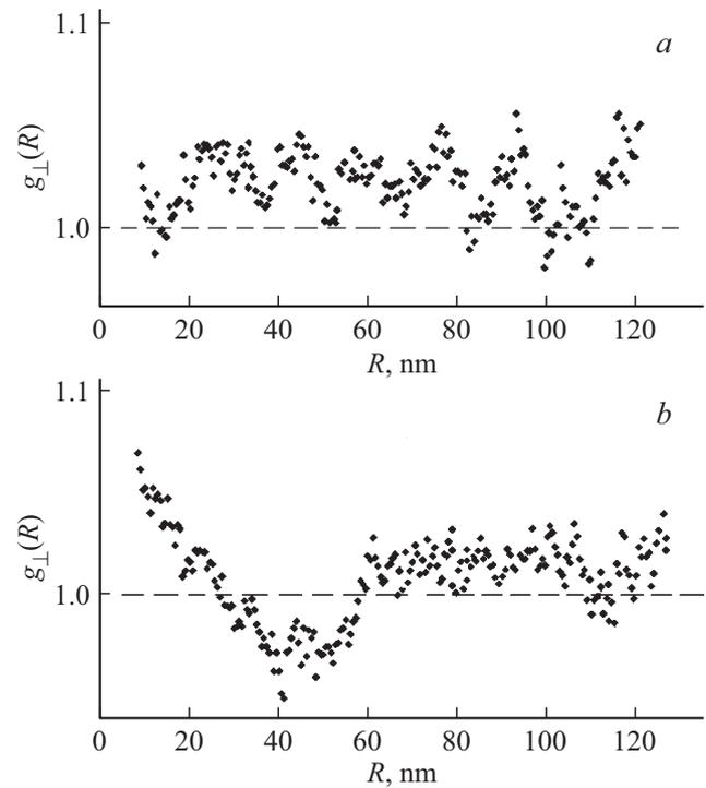
**Figure 5.** Radial functions of density distribution built across the axis of axial texture on the surface of CTA films: specimen № 1 (*a*), specimen № 2 (*b*). Step of surface image scanning  $\delta = 1$  nm.
