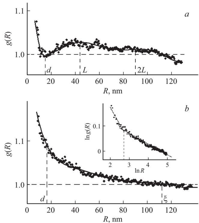
**Figure 3.** „Coarse-grained“ radial functions  $g(R)$  of gold nanoparticles distribution on the decorated replicas from the surface of CTA films (correlation functions  $g(R)$  of „density-density“ type): specimen № 1 (a), specimen № 2 (b). Step of surface image scanning  $\delta = 6$  nm. In the insert:  $g(R)$  function in double logarithmic coordinates for specimen № 2.
