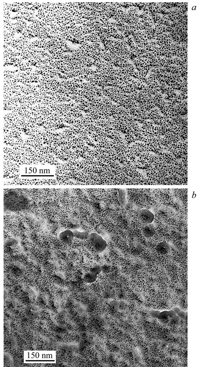
**Figure 1.** Electronic microphotos of gold-decorated germanium-carbon replicas from the surface of CTA films: specimen № 1 (a), specimen № 2 (b).
