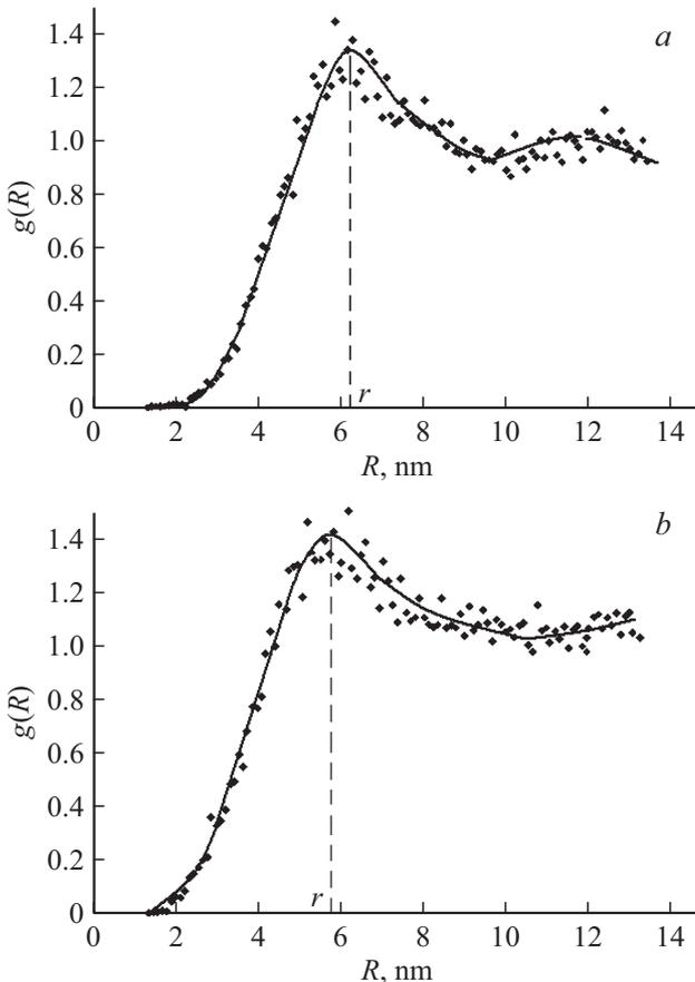
**Figure 2.** Radial functions  $g(R)$  of gold nanoparticles distribution on the decorated replicas from the surface of CTA films: specimen № 1 (a), specimen № 2 (b). Step of surface image scanning  $\delta = 1$  nm.
