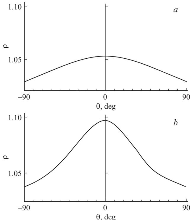
**Figure 4.** Indicatrices of relative (in relation to the mean value over the surface) density  $\rho$  of gold nanoparticles distribution on the decorated replicas from the surface of CTA films: specimen № 1 (*a*), specimen № 2 (*b*). Axis of the ordinates ( $\theta = 0$  degrees) corresponds to the texture axis — the direction with maximum value of  $\rho$ .
