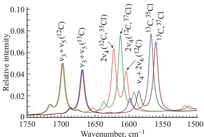
**Figure 4.** Superposition of calculated IR spectra of four  $\text{CHF}_2\text{Cl}$  isotopologues in the range of  $1750\text{--}1500\text{ cm}^{-1}$ . Color symbols:  $^{12}\text{C}, ^{35}\text{Cl}$  — red,  $^{12}\text{C}, ^{37}\text{Cl}$  — green,  $^{13}\text{C}, ^{35}\text{Cl}$  — blue,  $^{13}\text{C}, ^{37}\text{Cl}$  — brown.
