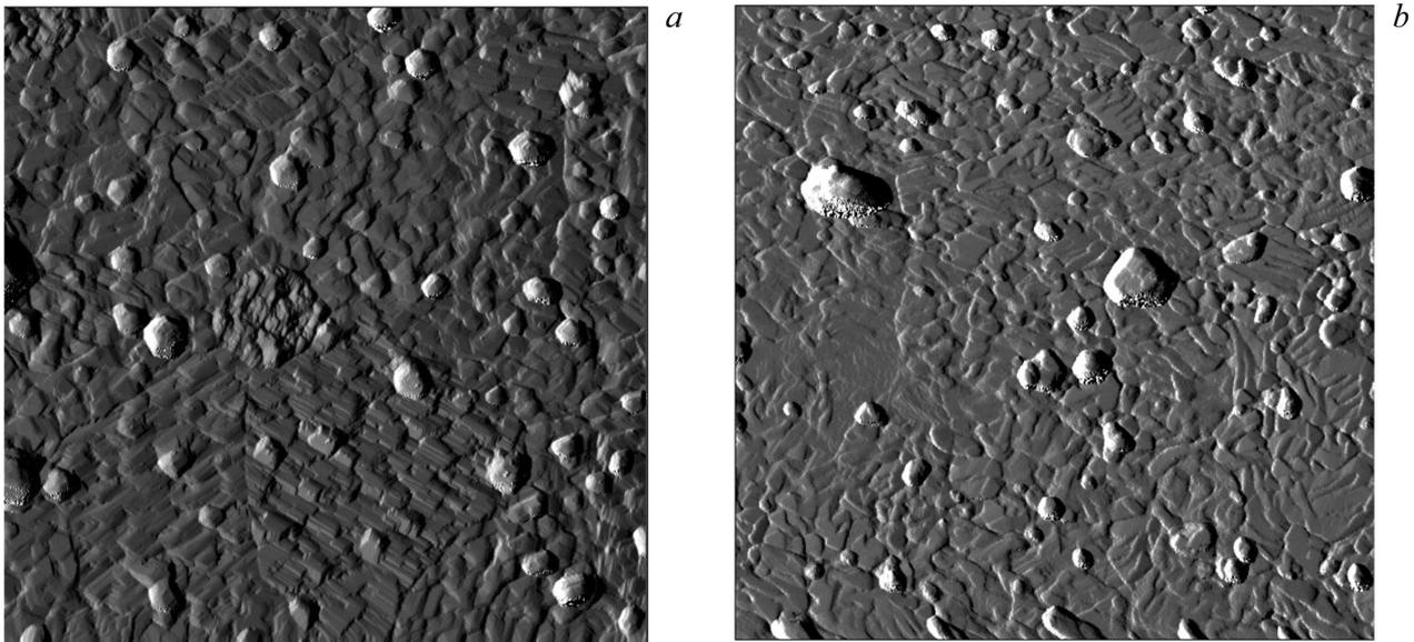
**Figure 1.** AFM-image of the surface of thin film (a)  $\text{Bi}_{95}\text{Sb}_5$  1  $\mu\text{m}$  thick on a underlayer of antimony 10 nm, (b)  $\text{Bi}_{92}\text{Sb}_8$  0.5  $\mu\text{m}$  thick on underlayer of antimony 10 nm. Image size is 10  $\times$  10  $\mu\text{m}$ .
