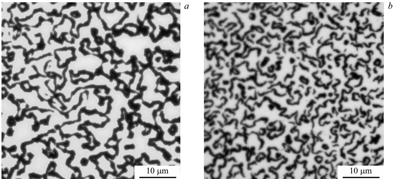
**Figure 2.** Micrograph of surface of thin film  $\text{Bi}_{97}\text{Sb}_3$  with thickness of  $0.5\ \mu\text{m}$  after chemical etching (a) without antimony underlayer, (b) on antimony underlayer  $10\ \text{nm}$ . The image size is  $50 \times 50\ \mu\text{m}$ .
