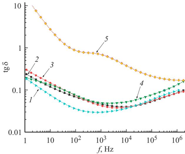
**Figure 4.** Dependence of a tangent of angle of dielectrical losses of chitosan films, containing 0 (1), 0.01 (2), 0.1 (3), 0.5 (4), 1.0 wt.% (5) SWCNT, on electric field frequency.
