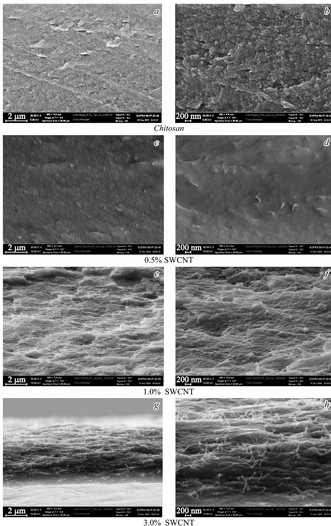
**Figure 2.** Microphotographs of shears in liquid nitrogen of chitosan film (*a, b*) and composite films, containing SWCNT (*c–h*).
