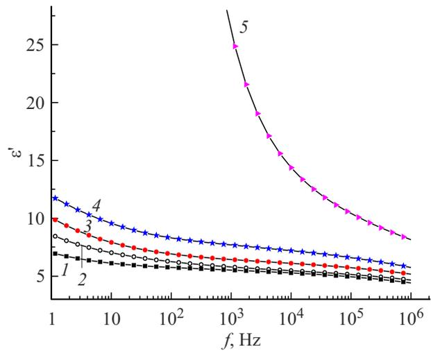
**Figure 5.** Dependence of relative permittivity of chitosan films, containing 0 (1), 0.01 (2), 0.1 (3), 0.5 (4), 1.0 (5) wt.% SWCNT, on electric field frequency.
