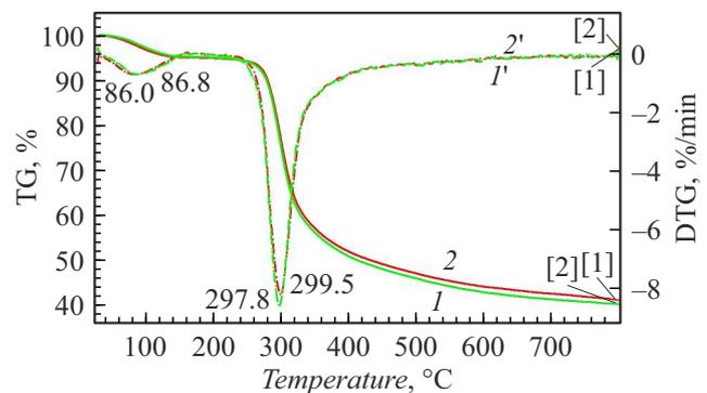
**Figure 6.** Thermogravimetric and differential thermogravimetric curves of the film of chitosan (1, 1') and composite film, containing 1 wt.% SWCNT (2, 2').
