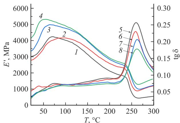
**Figure 7.** Dependence of elastic modulus  $E'$  of chitosan films, containing 0 (1), 0.5 (2), 1 (3), 3 (4) wt.% SWCNT, and the corresponding tangent of angle of mechanical losses (5–8) on temperature.
