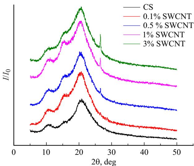
**Figure 1.** X-ray diffractograms of a film of chitosan (lower curve) and composite films with various SWCNT content (other curves).
