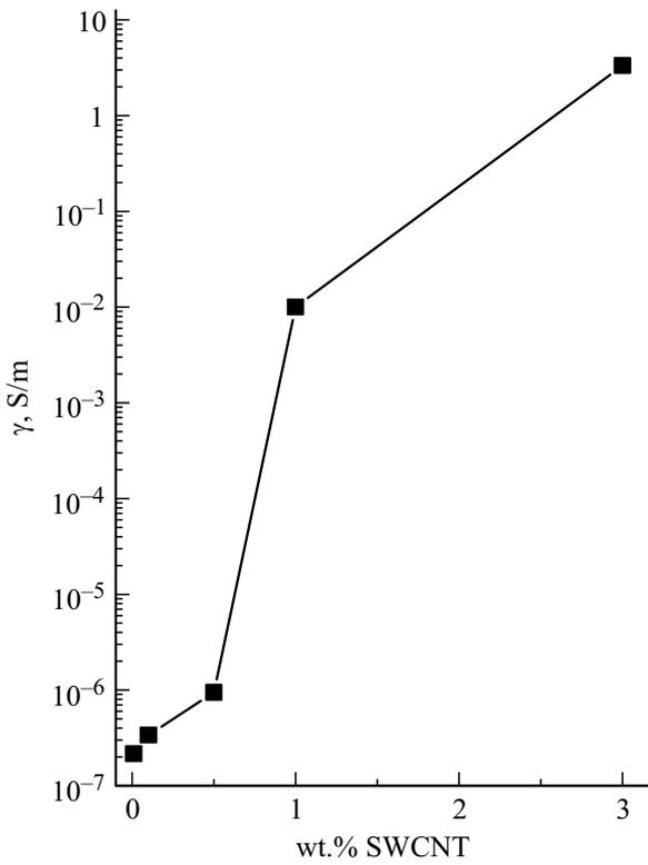
**Figure 3.** Change of volume electrical conductivity of composite films based on chitosan on SWCNT content.
