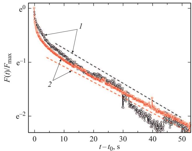
**Figure 4.** Combined relaxation dependences in semilogarithmic scale. 1 — switching  $U_{gate}$  at time  $t_0 = 18.8$  s, 2 — at time  $t_0 = 128$  s. Dashed lines are exponential dependences with time constant 31 (1) and 36 s (2). See text for explanation.
