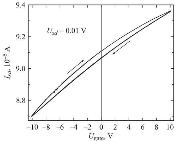
**Figure 5.** Gate characteristic with a sawtooth change  $U_{gate}$  with a sweep period 200 s is  $U_{sd} = 0.01$  V.
