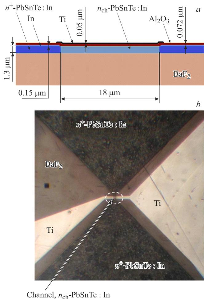
**Figure 1.** Schematic representation of the transistor-type MIS structure in the section (a) and photo of the finished experimental structure in the vicinity of the channel (b).
