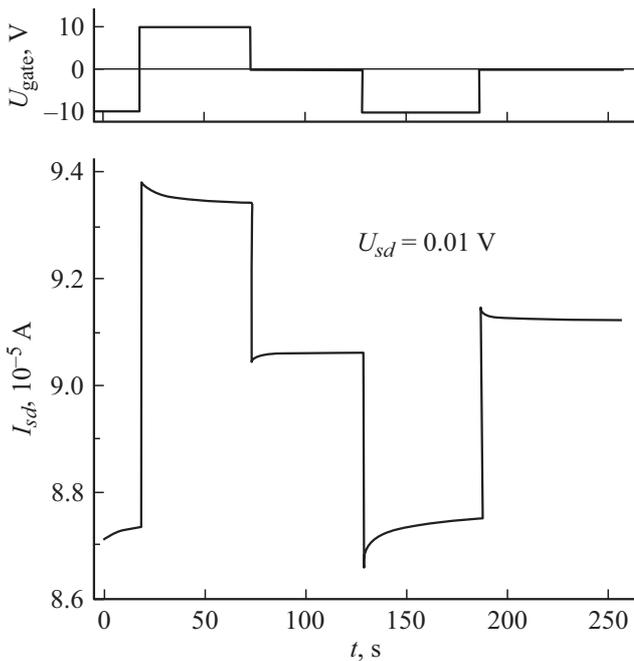
**Figure 3.** Current through channel of the MIS transistor  $I_{sd}(t)$  vs. time, and the corresponding dependence  $U_{gate}(t)$  at  $U_{sd} = 0.01$  V.
