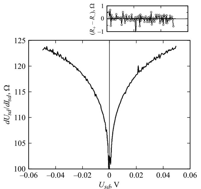
**Figure 2.** Numerically calculated from CVC the dependence of differential resistance of transistor-type MIS structure  $R = dU_{sd}/dI_{sd}$ . Top — difference  $(R_+ - R_-)$  between differential resistance at  $U_{sd} > 0$  and at  $U_{sd} < 0$  with equal absolute values  $U_{sd}$ .
