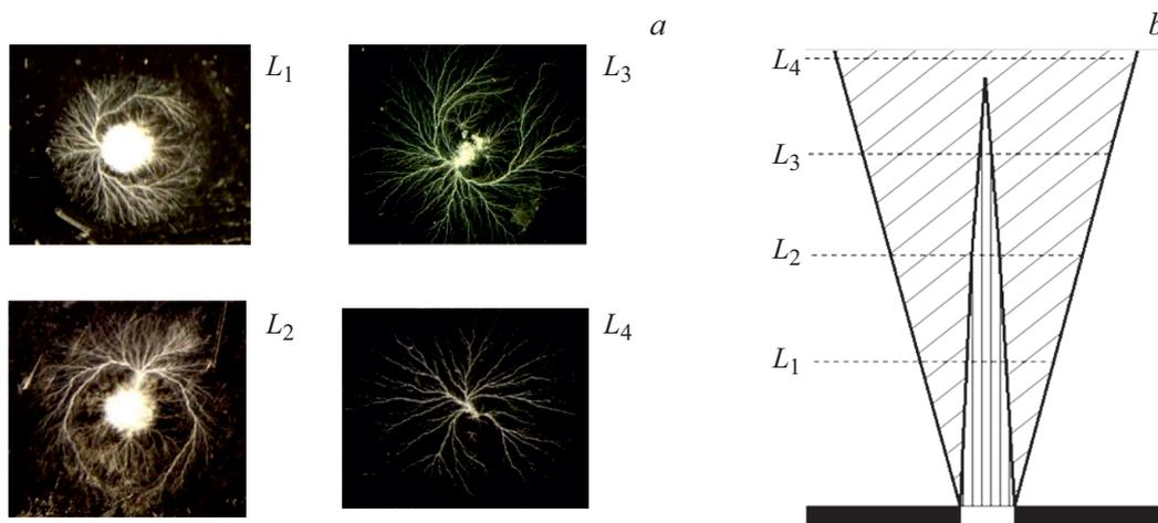
**Figure 1.** *a* — photographic images of PMMA destruction patterns produced by an electron beam output behind the anode of a vacuum diode at distance  $L_1 = 4$  mm,  $L_2 = 6$  mm,  $L_3 = 9$  mm, or  $L_4 = 13$  mm from the anode; *b* — spatial structure of electron beams output behind the anode of a vacuum diode.  $d_{CA} = 3.5$  mm,  $\varnothing_A = 1.5$  mm, and  $\varnothing_C = 6$  mm.
