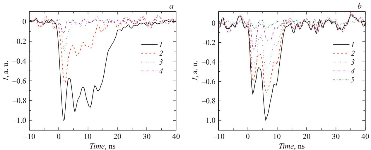
**Figure 2.** Oscilloscope records of current of the electron beam, which was output behind the anode of a vacuum diode, after its propagation through absorbing aluminum foils with a thickness of 30 (1), 80 (2), 130 (3), 230 (4), and 280  $\mu\text{m}$  (5). *a* — SFHCEB current, *b* — HEHCEB current.  $d_{CA} = 3.5$  mm,  $\varnothing_A = 1.5$  mm, and  $\varnothing_C = 6$  mm.
