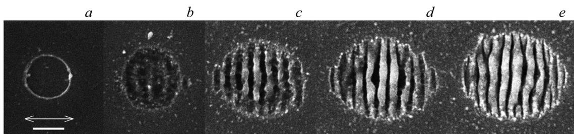
**Figure 6.** SEM image of multipulse craters 1030 nm. Pulse repetition rate is 5 Hz. Scale bar corresponds to  $2\ \mu\text{m}$ , the arrow shows the emission polarization. Pulse energy  $0.08\ \mu\text{J}$  — 1 pulse (a),  $0.08\ \mu\text{J}$  — 10 pulse (b),  $0.08\ \mu\text{J}$  — 30 pulses (c),  $0.08\ \mu\text{J}$  — 50 pulses (d),  $0.08\ \mu\text{J}$  — 100 pulses (e).
