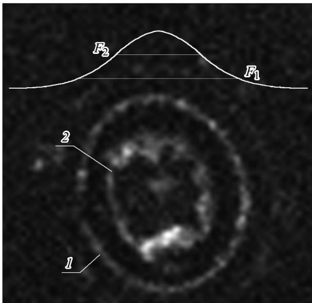
**Figure 3.** magnified image of a single-pulse crater for energy  $0.04 \mu\text{J}$ . 1 — spallation ablation crater boundary; 2 — molten region boundary; white line shows the laser pulse shape.  $F_1$  — spallation ablation threshold,  $F_2$  — melting threshold.
