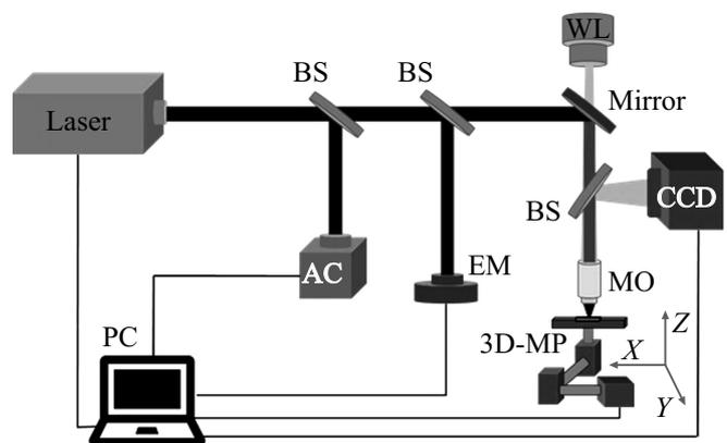
**Figure 1.** Fs/ps-laser ablation workstation setup: BS — beamsplitter, EM — energy meter, AC — autocorrelator, MO — microscope objective lens, WL — white-light source, PC — computer with preinstalled dedicated laser, camera, positioning system control software, CCD — camera for surface visualization during scanning.
