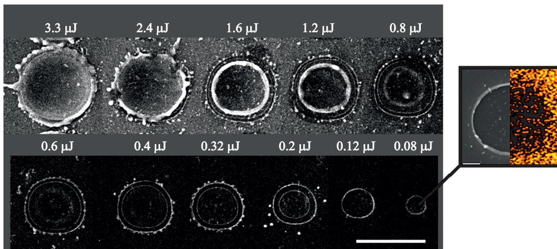
**Figure 5.** SEM image of single-pulse craters obtained at various energies and at 1030 nm. Scale bar corresponds to  $10\ \mu\text{m}$ . Detail: combined SEM/EDX image of single-pulse crater obtained at  $0.08\ \mu\text{J}$ . Scale bar corresponds to  $2\ \mu\text{m}$ . Yellow dots denote titanium particles.
