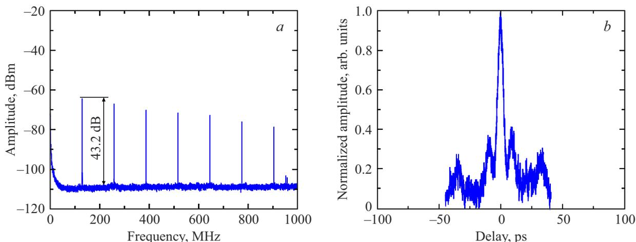
**Figure 3.** RF spectrum (a) and intensity autocorrelation (b) for the single-pulse mode (transmission of the resonator output mirror 5%).
