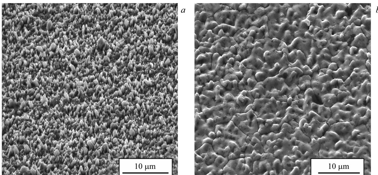
**Figure 2.** SEM images of the nanostructured nickel after irradiation with 30 keV argon ions and subsequent heating in vacuum with keeping for 15 min at 500 (a) and 800°C (b). The shooting angle is 45°.
