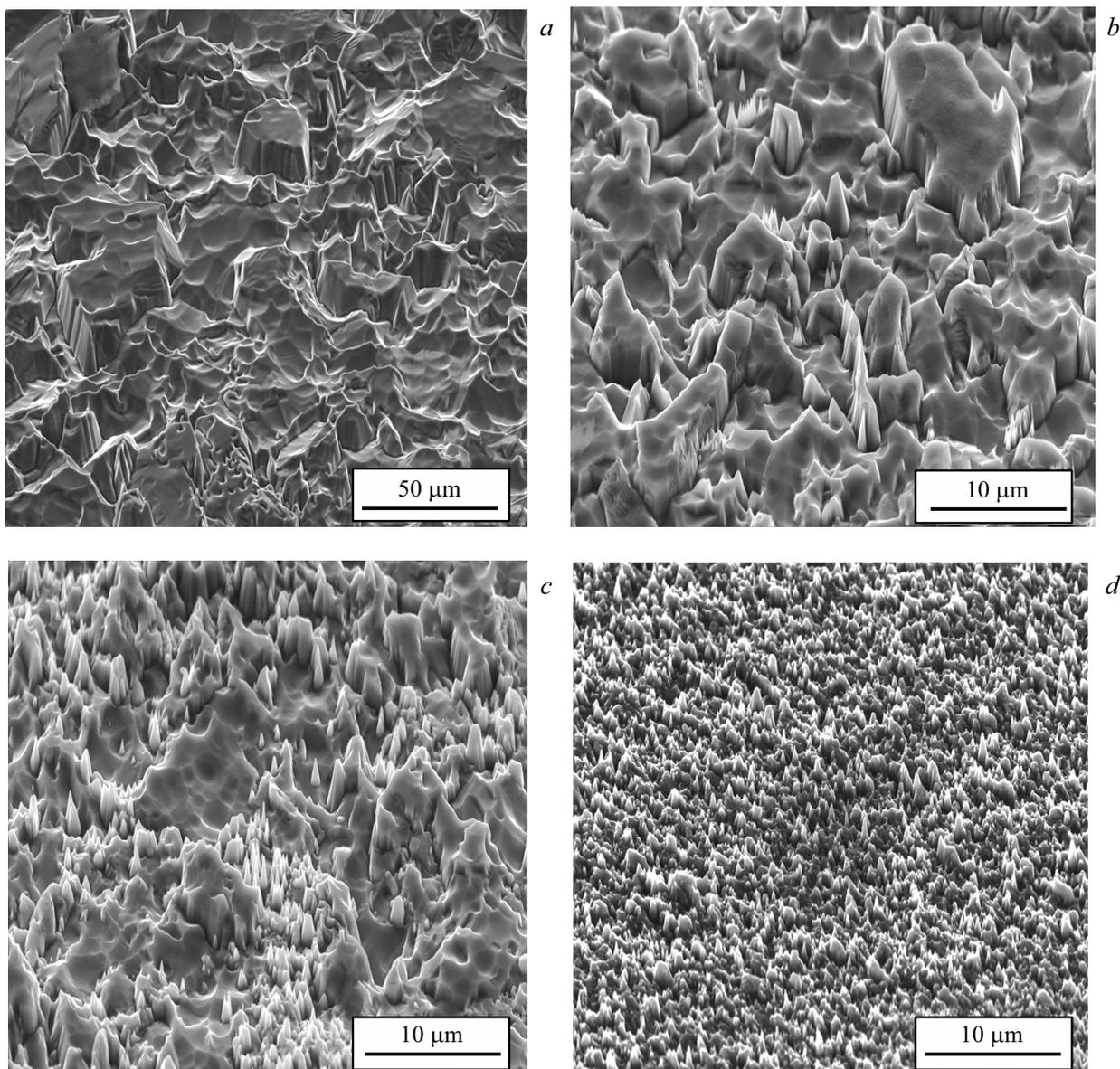
**Figure 1.** SEM images of the nickel surface with different grain sizes after high-fluence irradiation with 30 keV normally incident argon ions. Grain sizes (in  $\mu\text{m}$ ) were as follows: *a* — 30, *b* — 5, *c* — 2, *d* — 0.2. The shooting angle is  $45^\circ$ .
