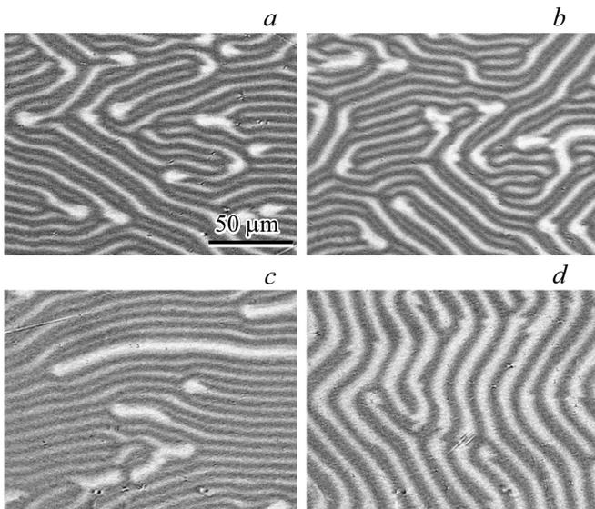
**Figure 6.** Images of the DS of the film FeNi(40 nm) as part of the YIG/FeNi (*a, b*) and YIG/Ta/FeNi (*c, d* systems) obtained in a zero field after magnetizing the samples to saturation along (*a, c*) and perpendicular to (*b, d*) the axis of the technological field. The measurement field application axis is parallel to the horizontal sides of the DS images.
