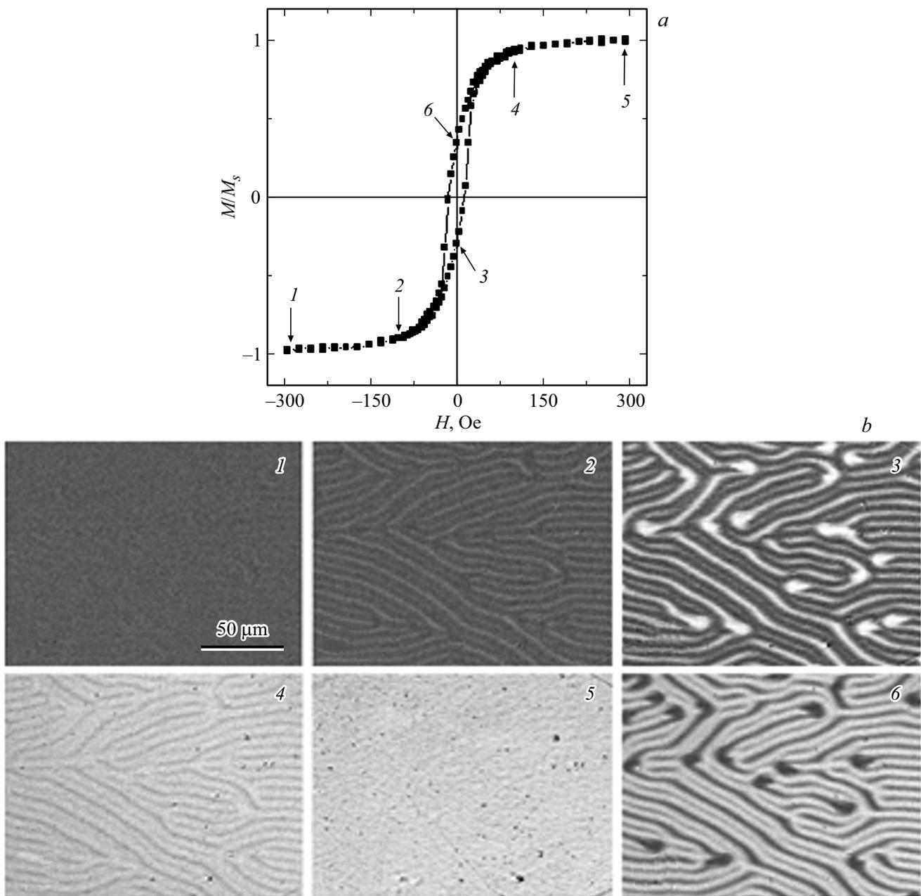
**Figure 4.** Magneto-optical hysteresis loop of the FeNi(40 nm) film deposited on YIG, measured in the geometry of the longitudinal Kerr effect along the axis of the technological magnetic field (a), and images of the magnetic domain structure corresponding to the sections of the loop hysteresis, indicated by numbers.
