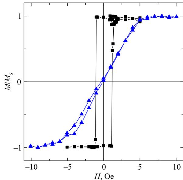
**Figure 3.** Magneto-optical hysteresis loops of the FeNi(10 nm) film, measured in the geometry of the longitudinal Kerr effect along (squares) and perpendicular (triangles) to the axis of the technological magnetic field.
