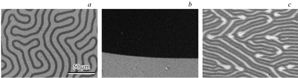
**Figure 2.** Images of the magnetic domain structure of the YIG (a), FeNi film on a glass substrate (b) and FeNi film deposited on YIG (c) obtained in the geometry of the polar (a) and longitudinal (b, c) Kerr effect.
