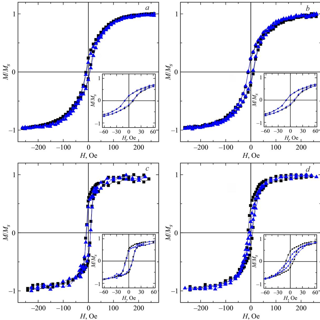
**Figure 5.** Magneto-optical hysteresis loops of 10 nm (*a, b*) and 40 nm (*c, d*) FeNi films deposited on YIG (*a, c*) and YIG/Ta(10 nm) (*b, d*) measured in the sample plane in the geometry of the longitudinal Kerr effect along (squares) and perpendicular (triangles) to the axis of the technological field. The insets show zoomed parts of the loops.
