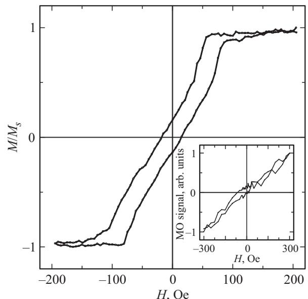
**Figure 1.** Magneto-optical hysteresis loops of the YIG film measured in the geometry of the polar Kerr effect when the magnetic field is oriented perpendicular to the sample plane and in the sample plane (inset).
