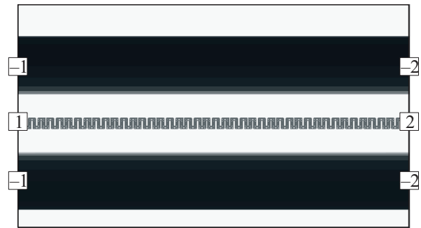
Figure 3. Current distribution in the Josephson contacts embedded in the coplanar transmission line.
