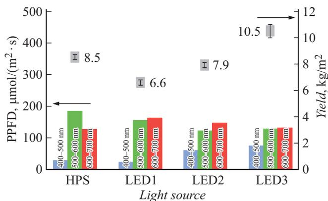
**Figure 5.** Productivity of tomato plants grown under light sources with different spectral composition.
