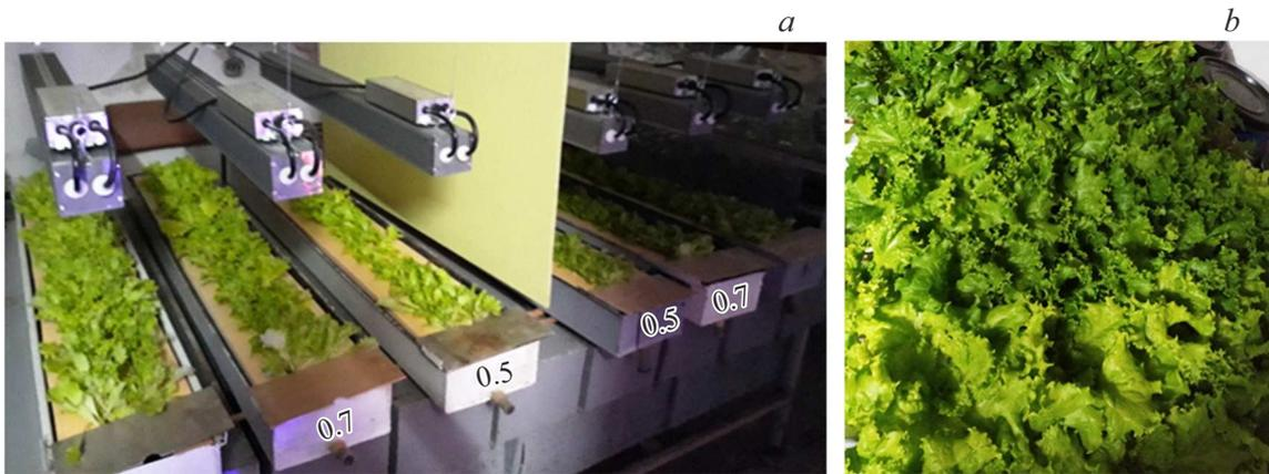
**Figure 2.** General view of experimental vegetation lighting systems with lettuce plants: *a* — under LED light sources, *b* — under HPS lamps.
