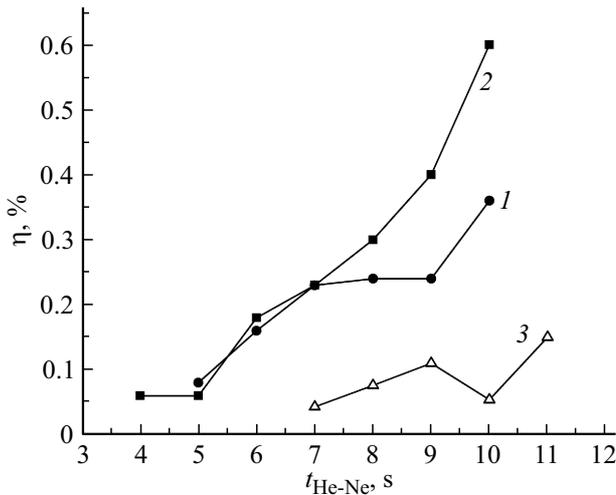
**Figure 1.** Dependence of the DE of  $\eta$  of primary holographic gratings on the time of exposure to He–Ne laser radiation for three options for processing a silver halide emulsion before UV exposure and etching: 1, 2 — direct rehalogenating bleaching, 3 — reversal whitening.
