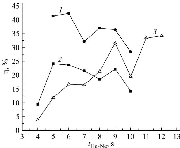
**Figure 2.** Dependence of DE of relief-phase holographic gratings on the time of exposure to He–Ne laser radiation for three options for photoemulsion processing after exposure to UV radiation and etching: 1, 3 — etching in the GAA solution (50%) + IPA (50%), 2 — etching in water.
