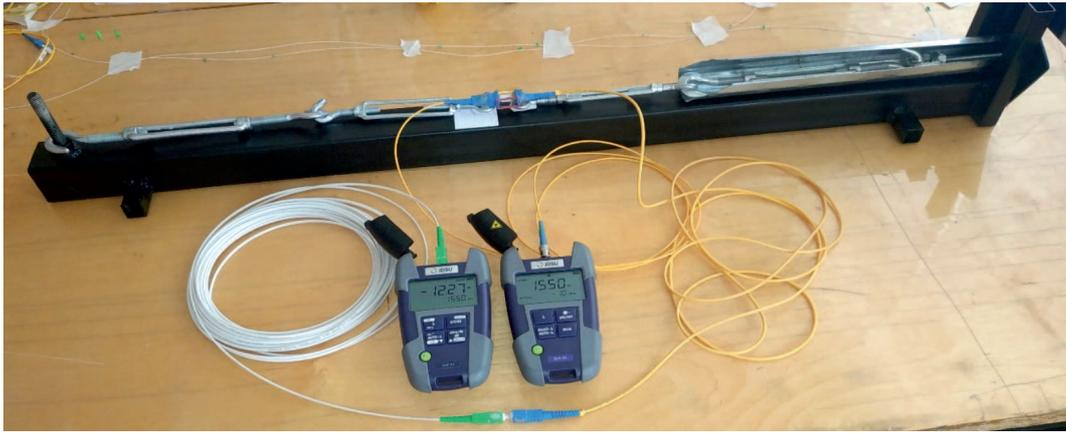
**Figure 2.** Photo of FOS prototype.
