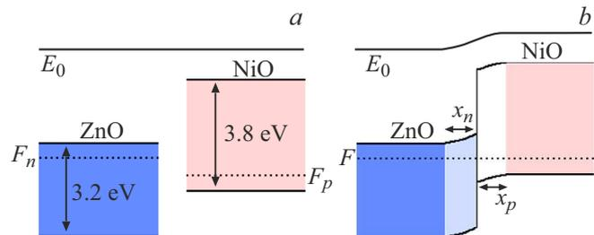
**Figure 3.** Energy band diagram of ZnO and NiO before (*a*) and after (*b*) contact.
