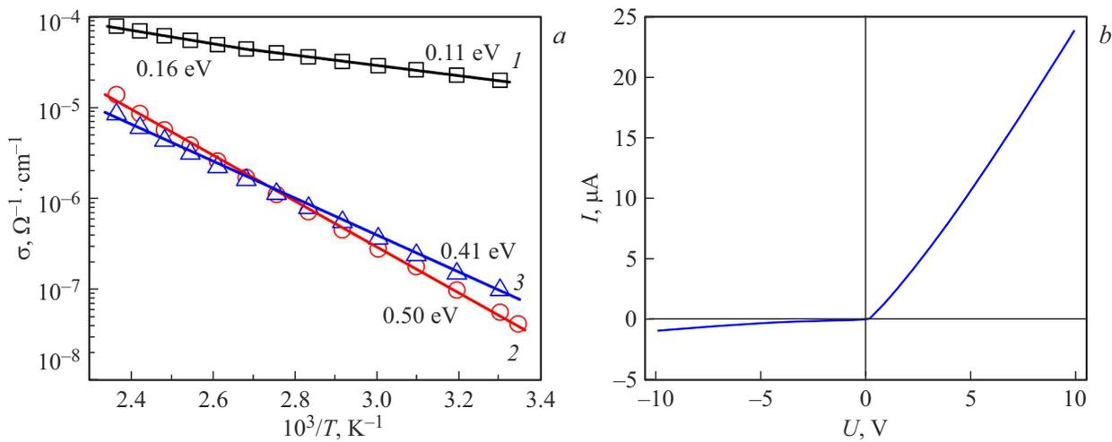
**Figure 2.** *a* — Temperature dependences of conductivities of ZnO (1), NiO (2), and composite I (3); *b* — current–voltage curve of composite II.
