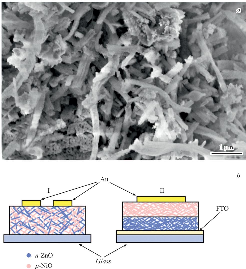
**Figure 1.** *a* — SEM image of composite I; *b* — schematic diagram of arrangement of composites I and II.
