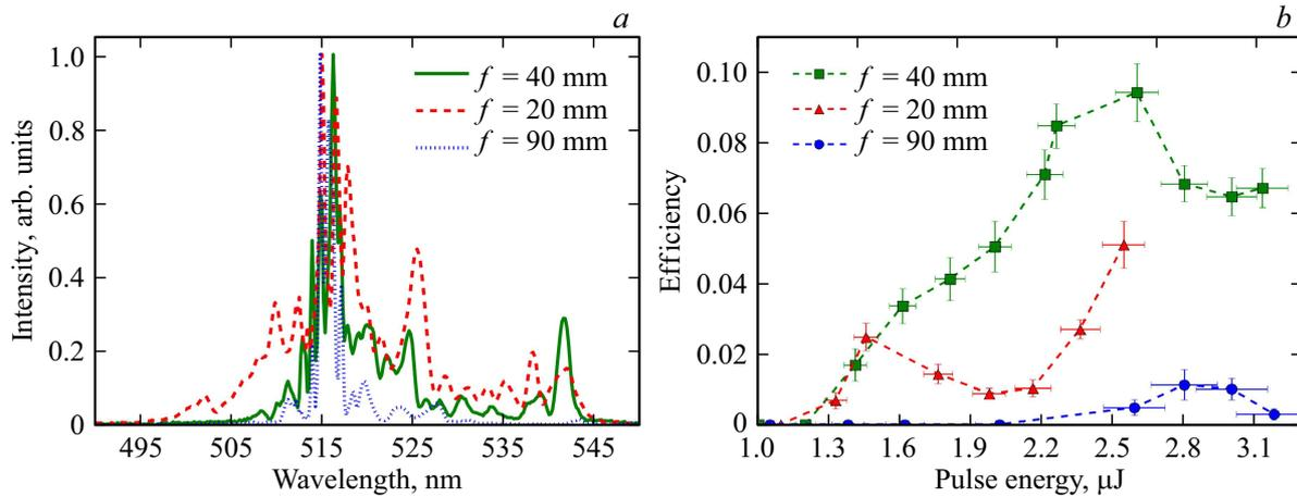
**Figure 2.** (a) Spectra of the emission passing through BWO crystal with maximum SRS component generation efficiency  $925\text{ cm}^{-1}$  at  $z = 0$  mm and various focusing lengths:  $f = 20, 40$  and  $90$  mm. (b) SRS component generation efficiency  $\nu_1 = 925\text{ cm}^{-1}$  of BWO crystal depending on the pulse energy at  $f = 20, 40$  and  $90$  mm.
