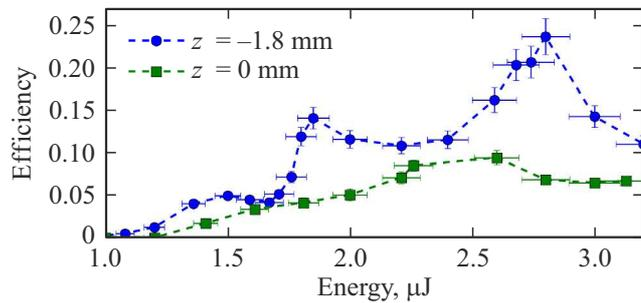
**Figure 4.** Dependence of generation efficiency of mode  $925\text{ cm}^{-1}$  for two positions ( $z = 0\text{ mm}$  and  $z = -1.8\text{ mm}$ ) on the laser pulse energy.
