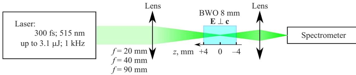
**Figure 1.** Optical scheme of the experiment. The  $z$  axis points out the linear focus position inside the crystal.
