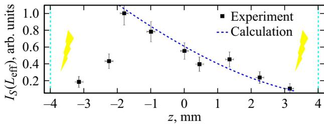
**Figure 3.** Dependence of the strongest SRS mode amplitude on the linear focus position inside the crystal. Dashes — calculation of conversion efficiency depending on the linear focus position taking into account varying filament length.
