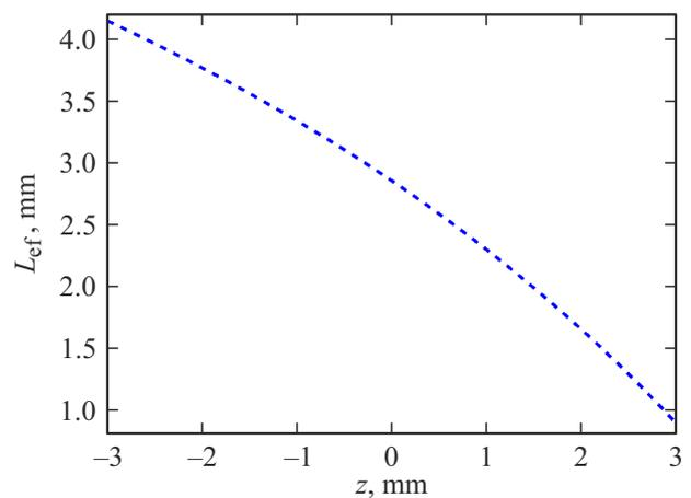
**Figure 5.** Calculated filament length from the linear focus position inside a  $8\text{ mm}$  long BWO crystal with laser pulse energy  $2.6\text{ }\mu\text{J}$ .
