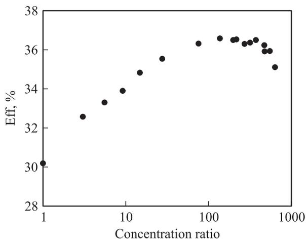
**Figure 4.** Efficiency of an InGaP/InGaAs/Ge concentrator 3-junction cell as a function of concentration ratio.
