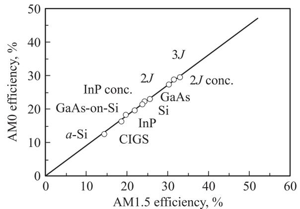
**Figure 7.** Correlation between AM0 and AM1.5 efficiencies for various solar cells.
