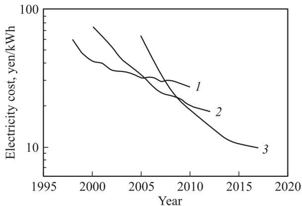
**Figure 6.** Scenario of electricity cost reduction by developing concentrator solar cells. The type of solar cell: 1 — Si-crystal, 2 — thin film, 3 — concentrator.
