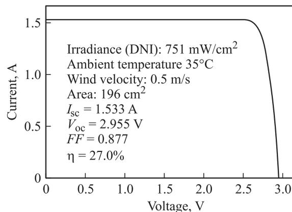
**Figure 5.** Outdoor evaluation of  $I - V$  with a plastic Fresnel lens (including loss in concentrator optics and temperature rise).
