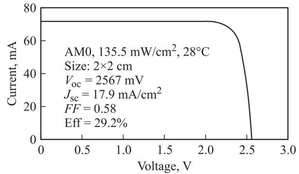
**Figure 2.** AM0  $I-V$  curve of InGaP/InGaAs/Ge 3-junction solar cell.
