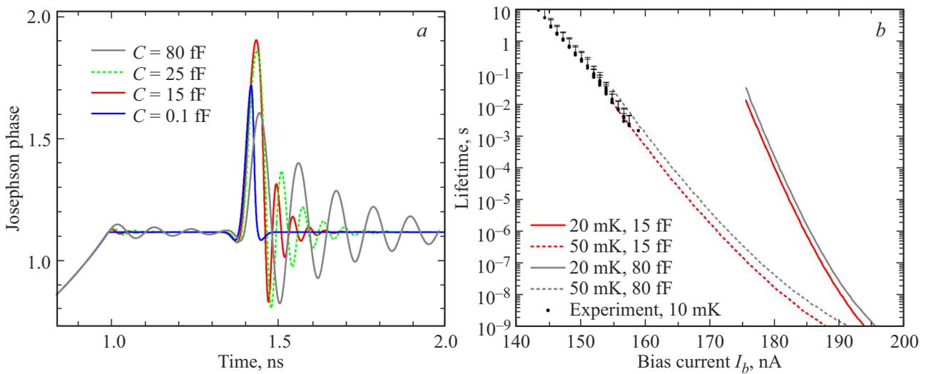
**Figure 3.** *a* — phase evolution after absorption of three 9 GHz photons with different capacitances. Case without fluctuations. *b* — life time for the best capacitance of 15 fF as simulated and technologically available capacitance of 80 fF at 20 and 50 mK. Black markers are experimental data for JJ with similar parameters and cryostat temperature 10 mK.
