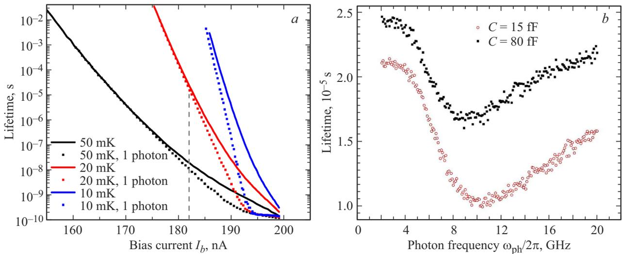
**Figure 4.** *a* — simulation of JJ life time with capacitance 80 fF at 50, 20 and 10 mK. Lines — life time defined by thermal fluctuations, markers — life time during photon arrival at time point = 0. The dashed line shows the shift current for which the right curve was calculated. *b* — simulation of life time at 20 mK from the photon frequency for two JJ capacitances. Shift current 182 nA.
