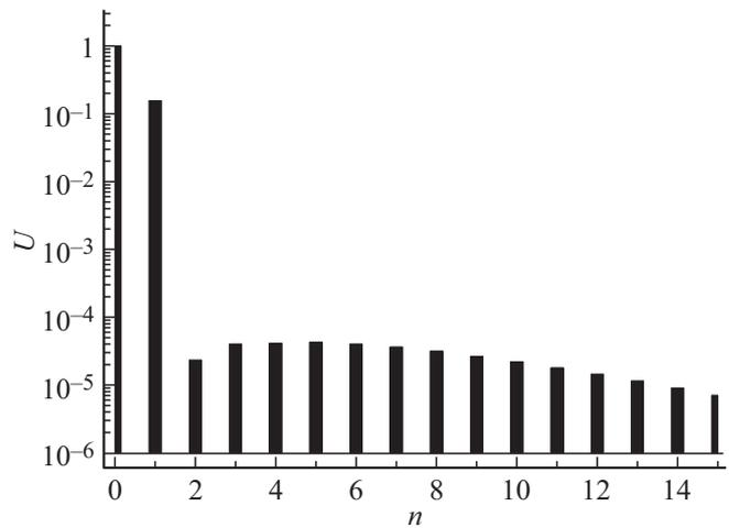
**Figure 3.** Voltage spectrum of the Josephson junction in pulse-frequency irradiation with shift current  $I = 1$  and modulation coefficient  $M = 40$  ( $\omega_0 = 1$ ).
