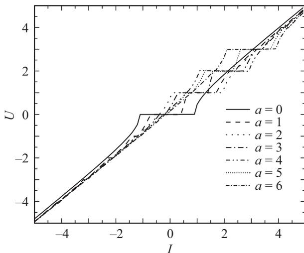
**Figure 2.** current-voltage curve at pulsed irradiation with various pulse amplitudes  $a$ . Modulation coefficient  $M = 0$ . Pulse repetition rate  $\omega_0 = 1$ .
