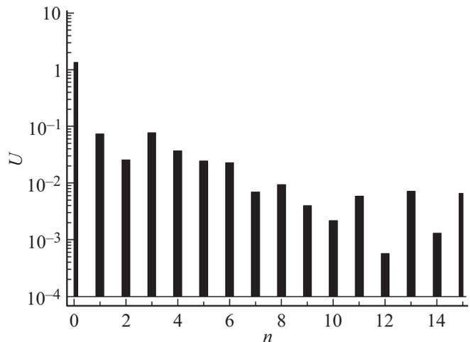
**Figure 4.** Voltage spectrum of the Josephson junction in pulse-frequency irradiation  $I = 2$  and modulation coefficient  $M = 40$  ( $\omega_0 = 1$ ).
