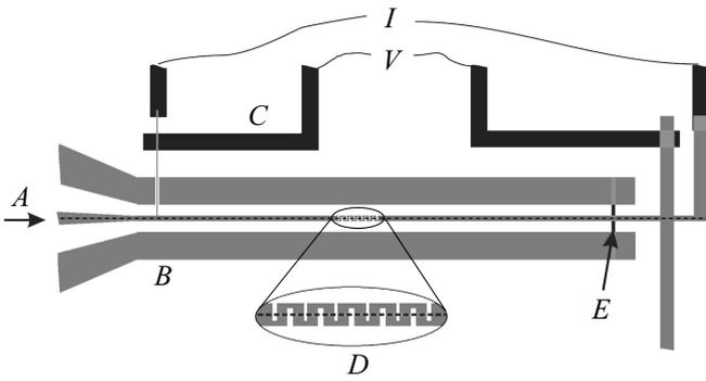
**Figure 1.** Photo pattern for the Josephson junction array made from high-temperature superconductors built in a coplanar transmission line. (A is the microwave power, B is the YBCO/Au coplanar transmission line, C are the NbN electrodes for passage of current and voltage measurement; D is the meander, E is the load). The dashed line shows the bicrystalline boundary.
