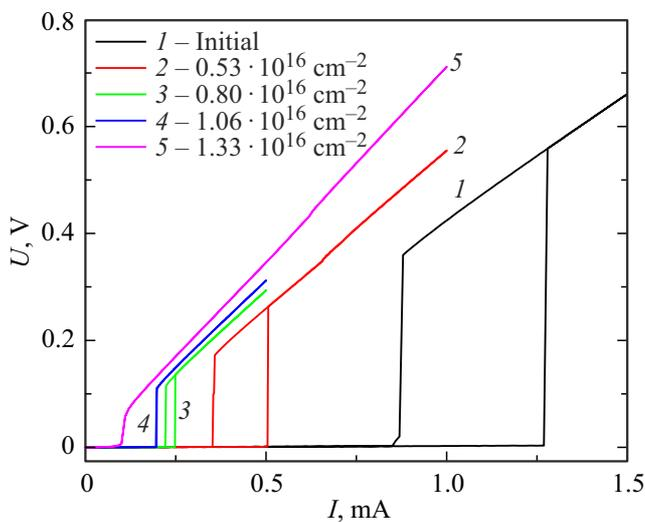
**Figure 2.** Current-voltage curves of the initial NbN film and after irradiation to some fluences and stabilizing annealing at 200°C.
