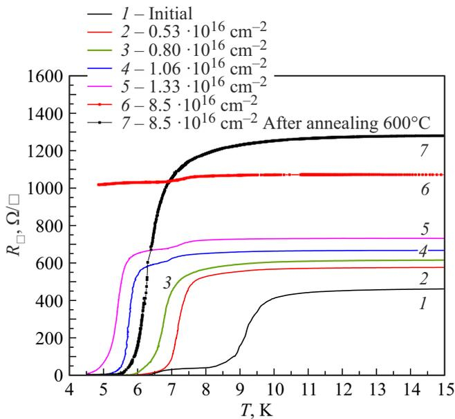
**Figure 1.** Dependence of resistance per square on temperature for initial NbN film and after irradiation and stabilizing annealing at 200°C.
