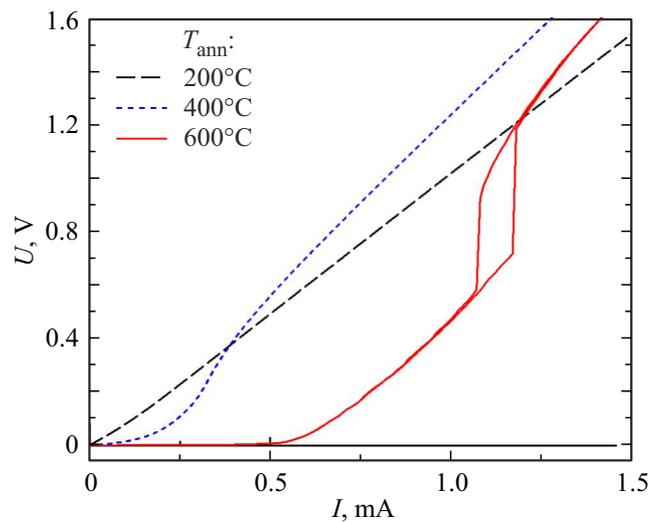
**Figure 3.** Current-voltage curves after irradiation to fluence  $8.5 \cdot 10^{16} \text{ cm}^{-2}$  and annealing at different temperatures.
