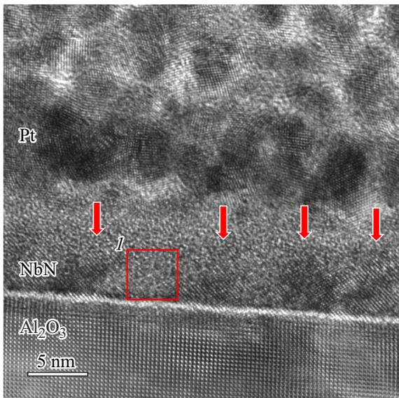
**Figure 4.** Electron-microscopic image of atom structure in the transverse cut of NbN film on a substrate of single-crystal sapphire after irradiation to fluence  $8.5 \cdot 10^{16} \text{ cm}^{-2}$  and annealing at temperature of  $600^\circ\text{C}$ : *I* — area between grains with loss of crystallinity (indicated with a square)
