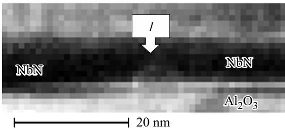
**Figure 5.** Chart of oxygen distribution in transverse cut of the NbN film after irradiation to fluence  $8.5 \cdot 10^{16} \text{ cm}^{-2}$  and annealing at temperature  $600^\circ\text{C}$ , produced by characteristic electron energy losses spectroscopy (EELS) method in the following mode: *I* — area between grains with higher oxygen content.
