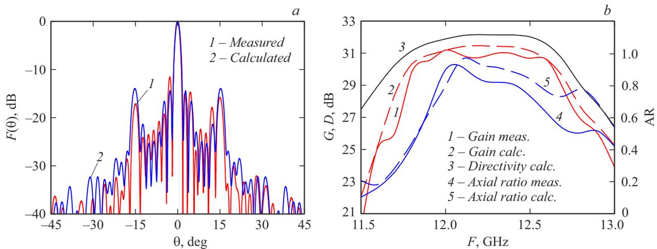
**Figure 3.** *a* — Measured and calculated directivity patterns of the antenna array in the horizontal plane; *b* — frequency dependences of the gain and the ellipticity.
