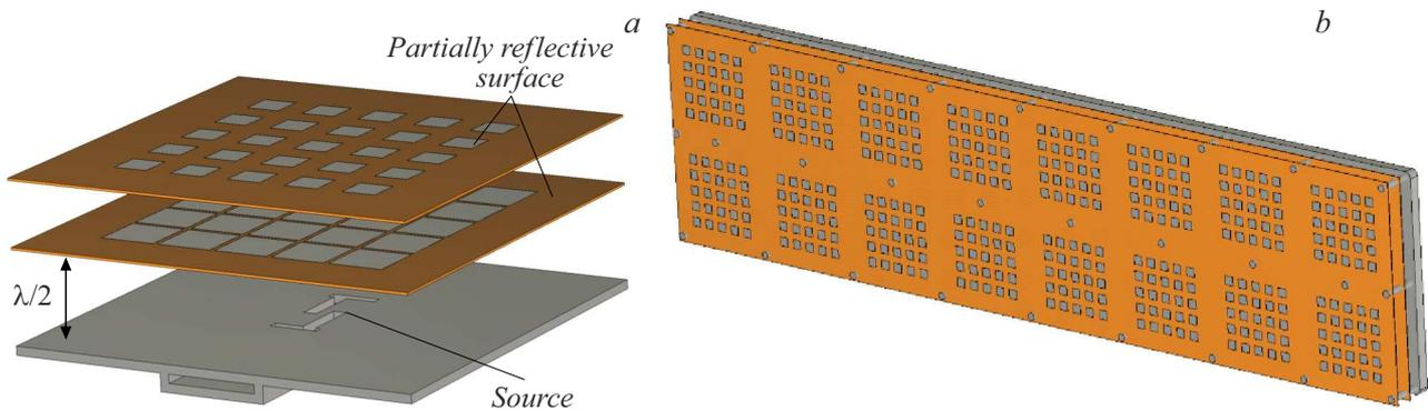
**Figure 1.** *a* — Structure of the Fabry–Pérot cavity; *b* — model of the antenna array based on Fabry–Pérot cavities.
