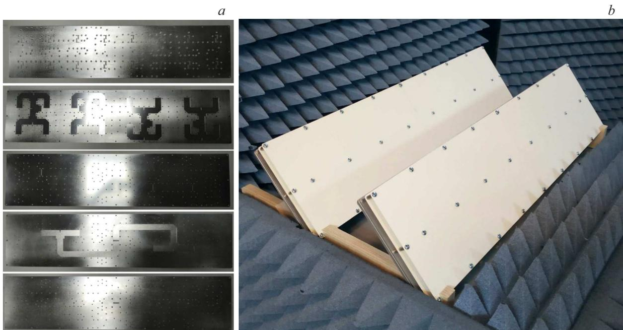
**Figure 2.** *a* — layers of the power divider of the antenna array; *b* — prototype models of antenna arrays based on Fabry–Pérot cavities.
