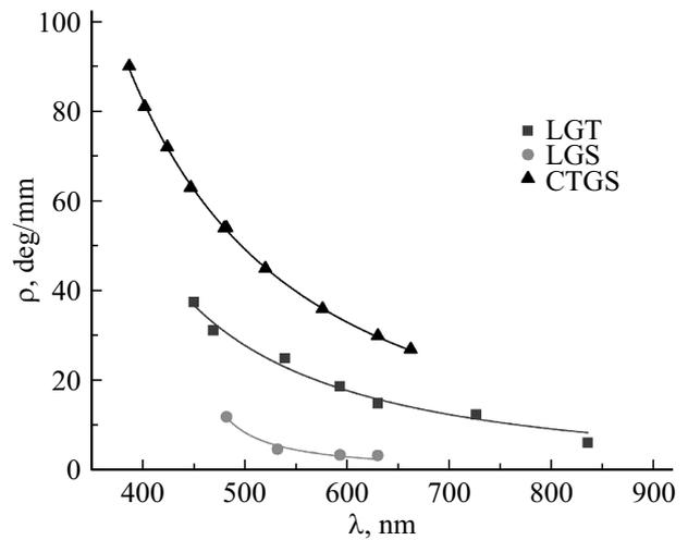
**Figure 4.** Dispersion dependences of the rotation angles of the polarization plane of LGS (circles), LGT (squares) and CTGS (triangles) crystals. The solid curves show the approximation dependences calculated by the Vyshin equation.
