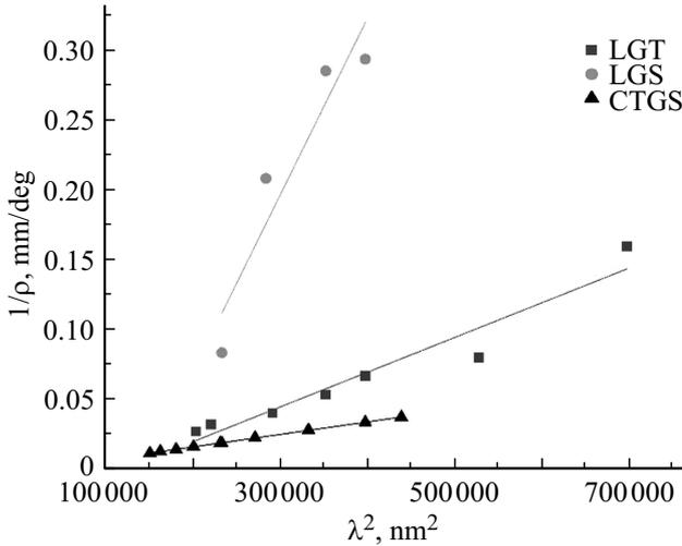
**Figure 5.** Dependences of the reverse specific rotation of the polarization plane on the squared wavelength of LGS (circles), LGT (squares) and CTGS (triangles) crystals. Solid curves show linear approximations.
