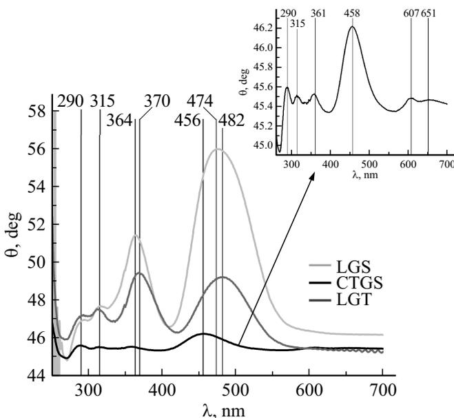
**Figure 3.** Spectral dependences of the transition dipole moment angles of LGS, LGT, CTGS crystals.
