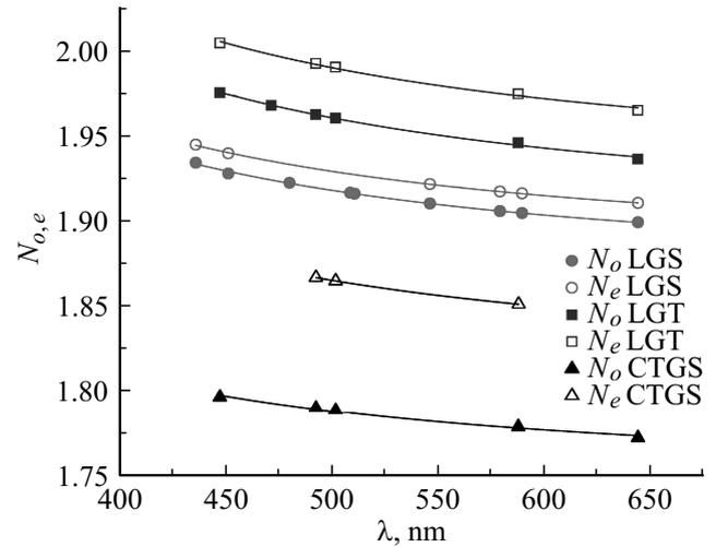
**Figure 6.** Dispersion dependences of the rotation angles of the polarization plane of LGS (circles), LGT (squares) and CTGS (triangles) crystals. The solid curves show the approximation dependences calculated using the Sellmeier equation.
