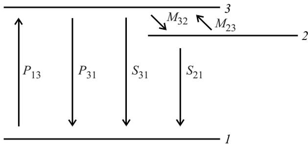
**Figure 1.** Diagram of population kinetics in a three-level atom.
