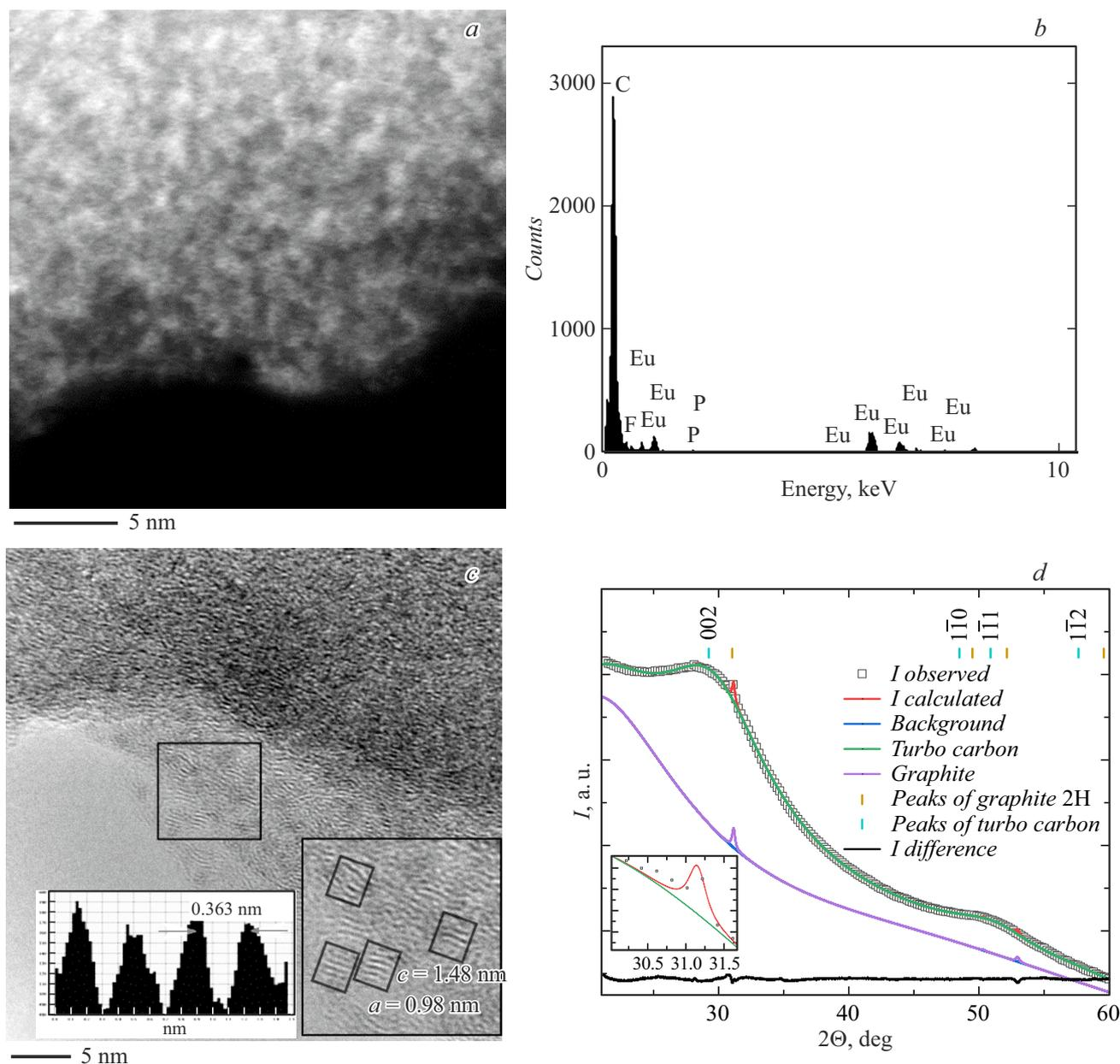
**Figure 2.** Analysis of pyrolyzed Eu diphthalocyanine by electron microscopy and X-ray diffraction analysis: dark-field mode of TSM (a); EDXS data (b); TEM bright-field mode (c); X-ray diffraction analysis (d).
