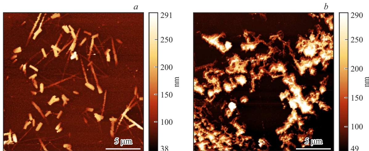
**Figure 1.** AFM image of morphology of  $\text{EuPc}_2$  (a) and its pyrolyzate (b) at  $800^\circ\text{C}$ .
