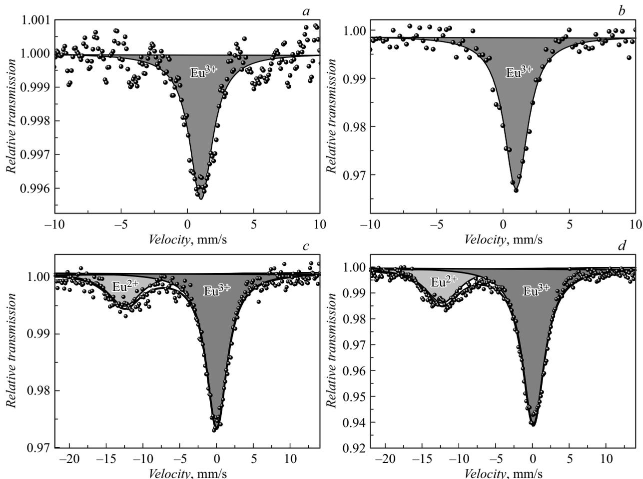
**Figure 3.** Mössbauer spectra of  $\text{EuPc}_2$  (a, b) and its pyrolyzate  $\text{EuPc}_2(\text{pyr})$  (c, d) at 300 and 80 K, respectively.
