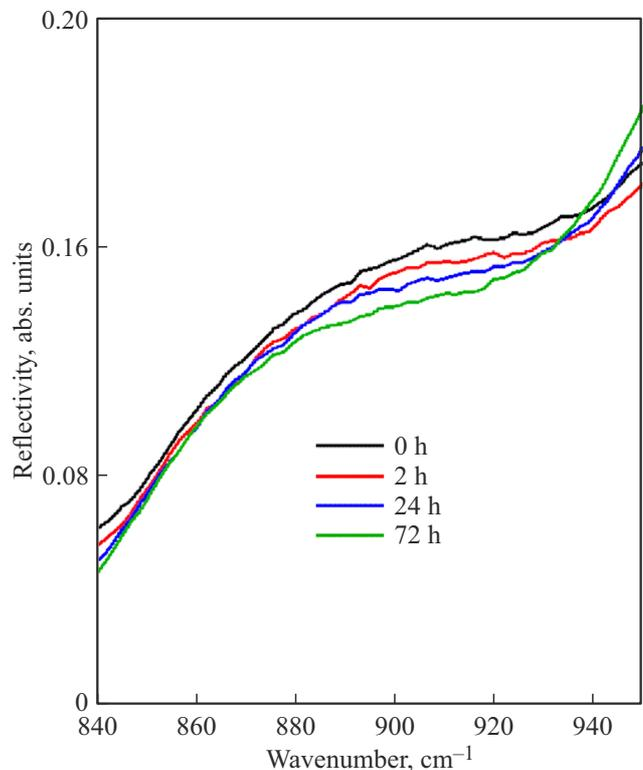
**Figure 2.** IR-spectrum of reflection in the area of band  $920\text{ cm}^{-1}$  before after the FA.
