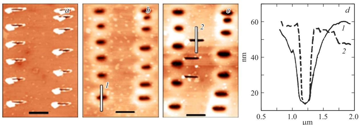
**Figure 5.** AFM images: *a* — mask in PMMA formed at room temperature and imaged prior to PMMA drying, relief height ( $\Delta h$ ) = 250 nm; *b* — the same mask after heating to 90°C (PMMA drying temperature), ( $\Delta h$ ) = 70 nm; *c* — the same mask with three new grooves cut in dried PMMA, ( $\Delta h$ ) = 140 nm. *d* — Height profiles along lines 1 and 2 (solid and dashed curves, respectively). The scale bar is 1.5  $\mu\text{m}$ .
