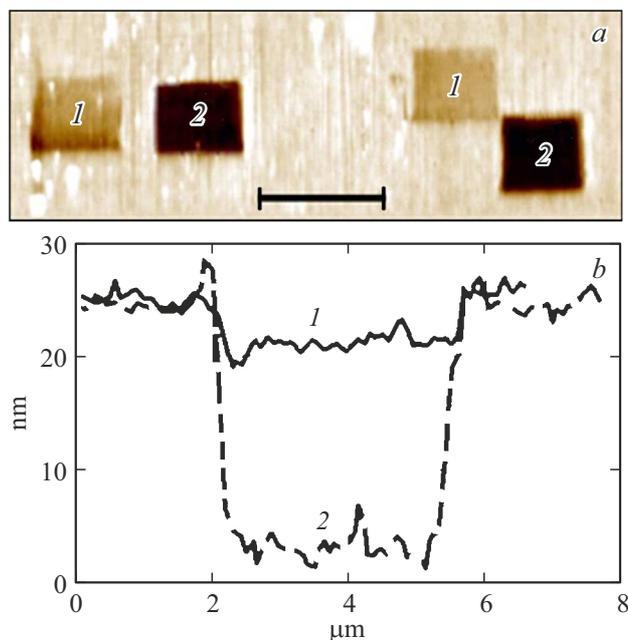
**Figure 6.** *a* — AFM image of the PMMA surface with certain regions of it subjected to one and the same pressing force at a sample temperature of 27°C (squares with number 1) and 55°C (squares with number 2). *b* — Height profiles for squares 1 (solid curve) and 2 (dashed curve). Squares were formed one after another at the corresponding temperatures. The scale bar is 5  $\mu\text{m}$ .
