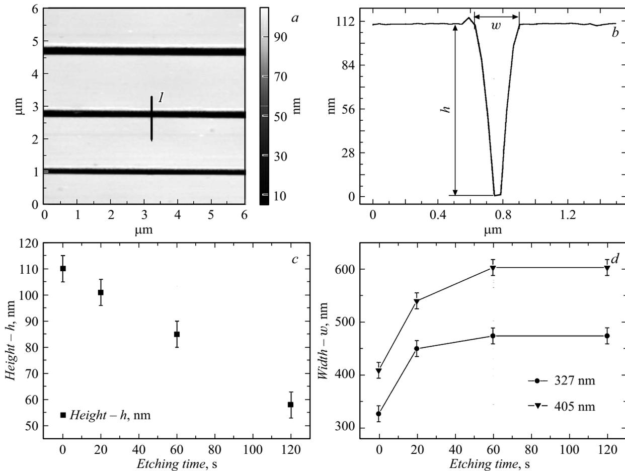
**Figure 7.** AFM image of a mask in PMMA (a) and profile along line *l* (b) that illustrates the parameters characterizing PMMA dissolution (width *w* of the formed groove and PMMA film thickness *h*). Dependence of the PMMA thickness (c) and the width of two grooves in PMMA with initial widths of 405 and 327 nm (d) on the time of etching with a developing solution.
