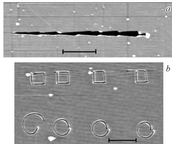
**Figure 3.** AFM images of a mask in PMMA in the form of a line (*a*) and contour figures (*b*) produced in the vector lithography mode in a single pass. The scale bar is  $5\ \mu\text{m}$ . Relief height: *a* — 100, *b* — 25 nm.
