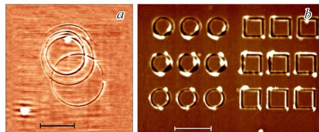
**Figure 4.** AFM images of a mask in PMMA formed in the vector lithography mode in several passes with capacitance sensors switched off (*a*) and on (*b*). The scale bar is  $4\ \mu\text{m}$ . Relief height: *a* — 14, *b* — 140 nm.
