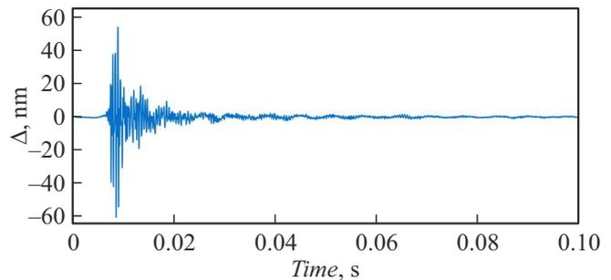
**Figure 5.** A finger-click signal next to the sensor interferometer.
