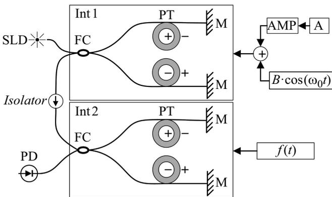
**Figure 1.** The scheme of the tandem interferometer (TI) assembled in the experiment. Notations: Int1 and Int2 — reference and sensor interferometer, respectively, SLD — superluminescent diode, FC — fiber optic splitter 2×2, PT — piezoceramic coils, M — Faraday mirror, Isolator — fiber-optic insulator, PD — photodetector, A — digital-to-analog converter, AMP — high-voltage amplifier,  $B \cdot \cos(\omega_0 t)$  — reference modulation,  $f(t)$  — measurable impact.
