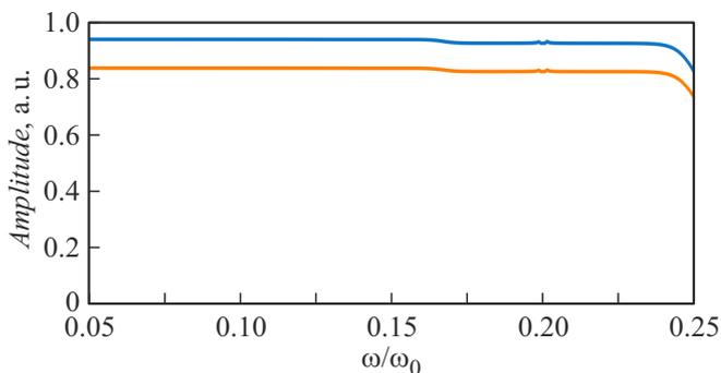
**Figure 2.** The calculated amplitude of the output signal of the proposed scheme at a constant input for precise adjustment of interferometers (blue curve (in the online version)) and for the case of a 4-band shift of the interference pattern (orange curve (in the online version)).
