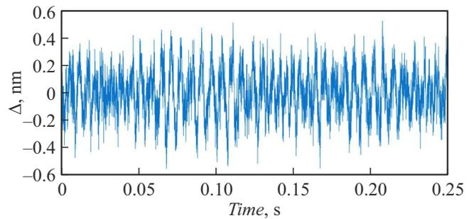
**Figure 4.** The noise track of the registration system, converted into nanometers.
