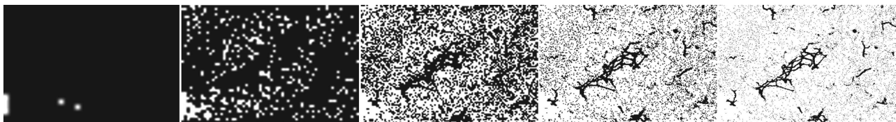
Figure 6. Successive local adaptive binarization frames of the SEM image of the Ni nanonetwork after 10 minute ablation.
