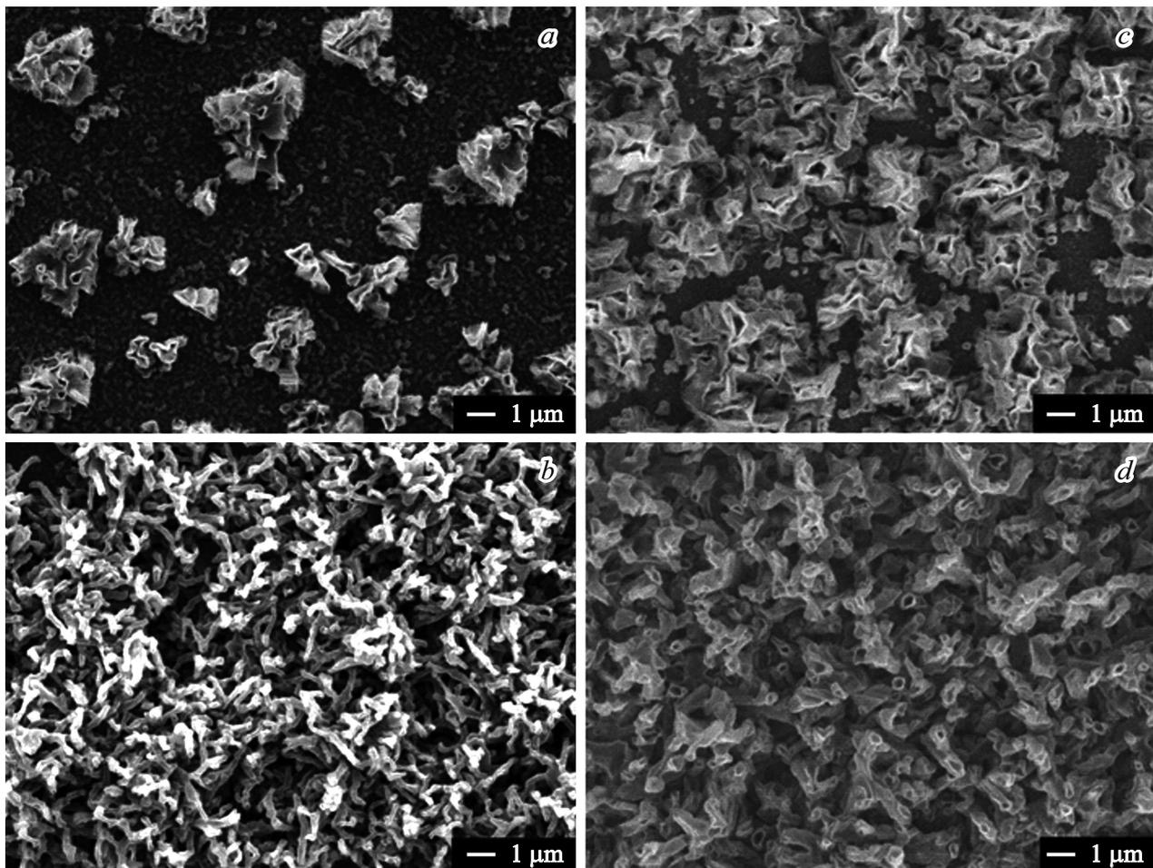
**Figure 4.** SEM-images of transferred SiC layers with nanotubes produced at: *a*) Si (111), *t* = 3.5 min, *b*) Si (111), *t* = 40 min, *c*) Si (100), *t* = 3.5 min, *d*) Si (100), *t* = 40 min.
