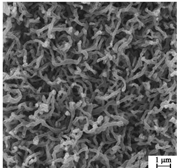
**Figure 2.** SEM-image of an inverted SiC layer with nanotubes transferred onto a LK5 glass substrate.
