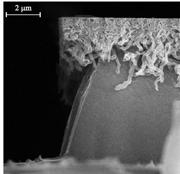
**Figure 1.** SEM image of the formed SiC nanostructures growing from the SiC layer downwards, i.e. „from top to bottom“.
