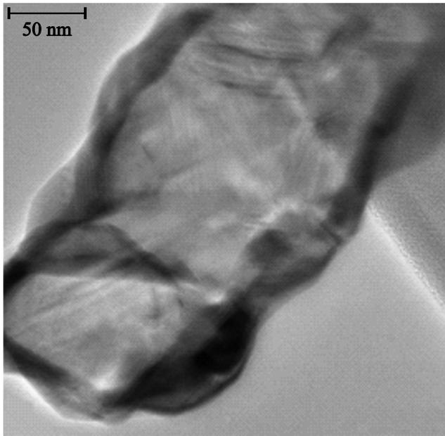
**Figure 3.** TEM-images of a single SiC nanotube.
