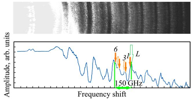
**Figure 3.** Interference pattern of the „forward“ scattered radiation obtained using the  $F-P$  interferometer (with the AltMV virus suspension in the cell). The dispersion region of the interferometer is 150 GHz. Hereinafter:  $L$  is laser emission line,  $1-6$  is numbering of Stokes lines (see the table for frequency detuning values).
