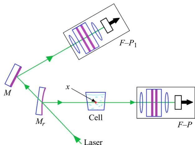
**Figure 1.** Schematic diagram of the measurements. Laser — direction of picosecond laser radiation; Cell — cell with the test substance;  $F-P$ ,  $F-P_1$  — Fabry-Perot interferometers with a registration system;  $M$  — totally reflecting plane mirror;  $M_r$  — spherical mirror ( $f \sim 12.5$  cm, reflectance is  $\sim 80\%$ )  $x$  — location of the focused laser beam waist in the middle of the cell.
