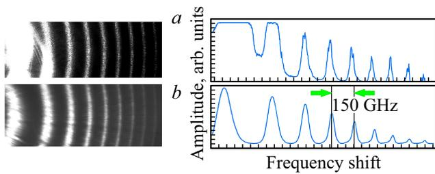
**Figure 2.** Interference patterns of the „forward“ scattered radiation obtained from the  $F-P$  interferometer (with buffer solution in the Cell —  $a$ ) and the  $F-P_1$  interferometer (laser emission spectrum  $b$ ). The dispersion regions of the interferometers are the same and equal to 150 GHz. Hereinafter: the bright spot in the interference pattern in Fig. 2,  $a$ , 3 and 4 is caused by illumination from the SRS component excited in the buffer liquid.
