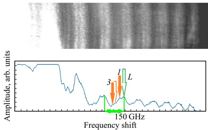
**Figure 4.** Interference pattern of the „forward“ scattered radiation obtained using the  $F-P$  interferometer (with the PVX virus suspension in the cell). The dispersion region of the interferometer is 150 GHz. Here  $1-3$  is numbering of Stokes lines.
