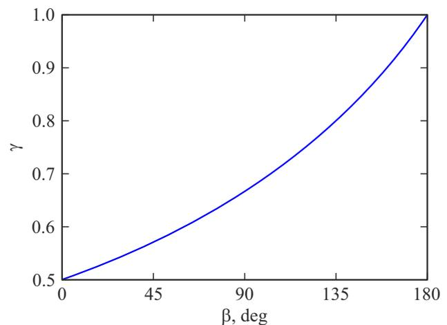
**Figure 2.** Dependence of the field inhomogeneity exponent  $\gamma$  on the opening angle of the wedge-shaped cathode  $\beta$ .
