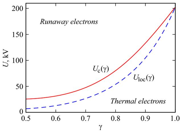
**Figure 3.** The threshold voltage for electron runaway as a function of the field inhomogeneity exponent  $\gamma$  (gas — atmospheric air at pressure 760 Torr and temperature 300 K,  $D = 7.5$  mm):  $U_c$  — numerical calculation,  $U_{loc}$  — local criterion (7).
