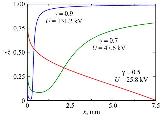
**Figure 4.** Distributions of the reduced force acting on the RAE  $f_n$  in the interelectrode gap for  $\gamma = 0.5, 0.7, 0.9$  at near-threshold voltage values  $U \approx 25.8, 47.6, 131.2$  kV respectively (gas — atmospheric air at pressure 760 Torr and temperature 300 K,  $D = 7.5$  mm).
