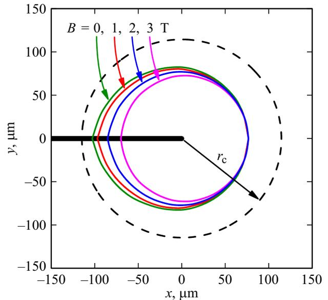
**Figure 6.** Runaway areas in the vicinity of the blade cathode apex for  $B = 0, 1, 2, 3$  T ( $U = 50$  kV,  $D = 7.5$  mm, gas — atmospheric air at pressure 760 Torr and temperature 300 K). The dashed line shows the area (circle of radius  $r_c \approx 114 \mu\text{m}$ ) in which the electric field strength exceeds the threshold  $E_c$ .
