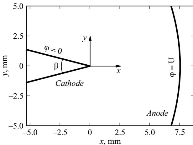
**Figure 1.** Geometry of the interelectrode gap for  $\beta = 30^\circ$  and  $D = 7.5$  mm
