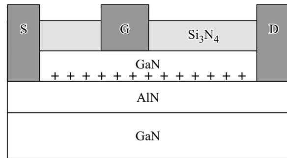
**Figure 1.** Design of *p*-channel Schottky gate transistor based on GaN/AlN/GaN heterostructure.
