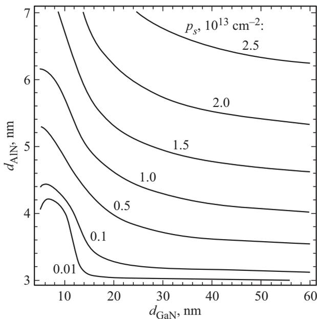
**Figure 2.** The dependence of the layer concentration  $p_s$  of a two-dimensional hole gas on the thicknesses of AlN stressed barrier layer ( $d_{\text{AlN}}$ ) and the strongly doped GaN layer ( $d_{\text{GaN}}$ ).
