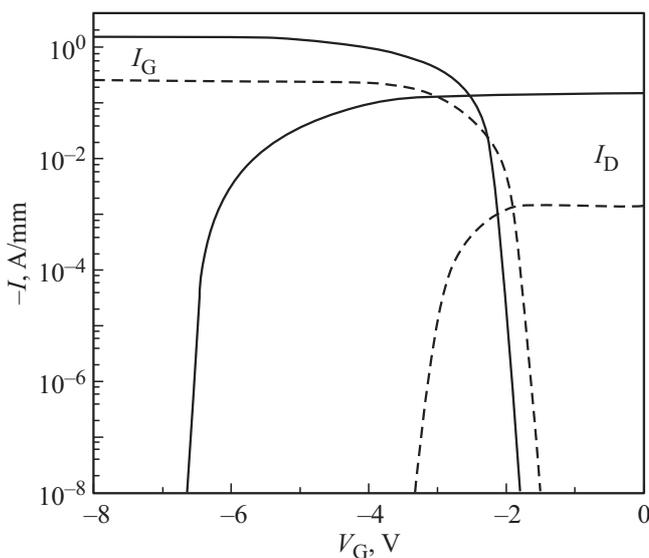
**Figure 3.** The dependence of the drain current ( $I_D$ ) and the gate current ( $I_G$ ) on the value of the gate-source voltage for transistors with AlN layer thickness of 5 nm (solid line) and 3 nm (dotted line).
