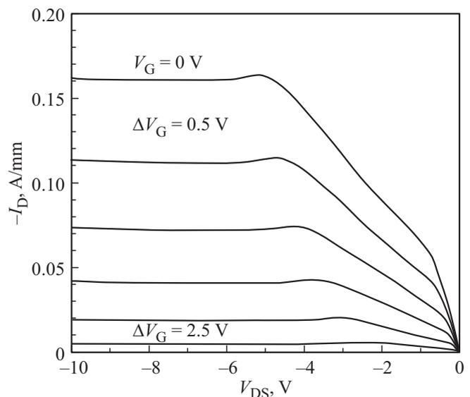
**Figure 6.** Output characteristics of a gate transistor in a two-dimensional electron gas layer.
