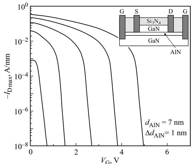
**Figure 5.** The dependence of the maximum drain current density at saturation on the gate voltage at different thicknesses of the AlN barrier layer in the range  $d_{AlN} = 3$ – $7$  nm.
