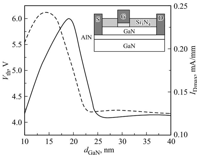
**Figure 4.** Dependence of the threshold voltage  $V_{th}$  (solid line) and the maximum drain current  $I_{Dmax}$  (dotted line) on  $n^+$ -GaN layer thickness.
