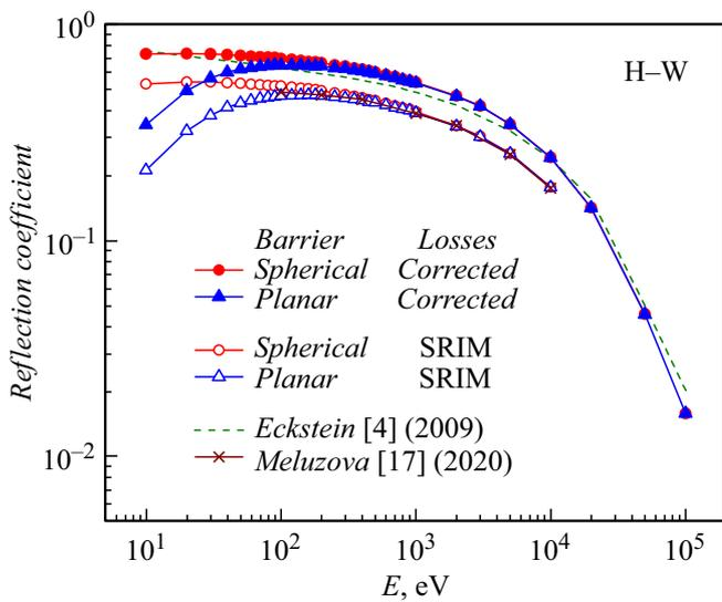
**Figure 4.** Reflection coefficients for H–W system. Calculation for two electronic stopping models is provided: SRIM package and dependence corrected for multiple collisions [35], for spherical and planar barriers. For comparison, Eckstein’s [4] and Meluzova’s [17] calculations are provided.
