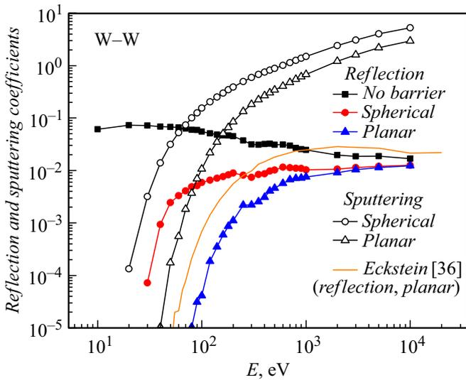
**Figure 3.** W–W system. Comparison of reflection and sputtering coefficients for spherical and planar surface barriers and for the case without a barrier (reflectance). The line shows the reflection coefficient calculation from [36] for the planar barrier case.
