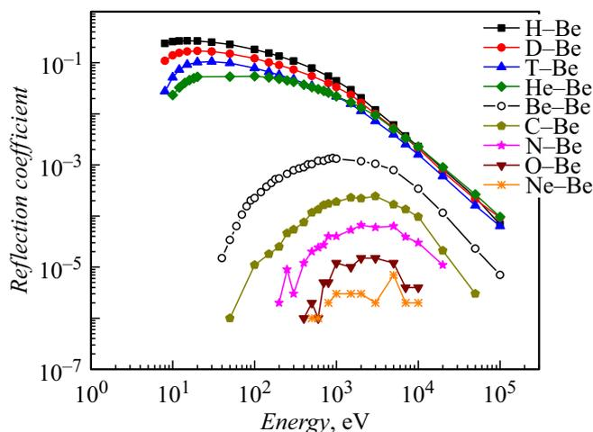
**Figure 1.** Calculated particle reflection coefficients on beryllium target depending on the energy for bombarding H, D, T, He, Be, C, N, O, Ne atoms. For Be–Be system, the planar potential barrier calculation is provided.
