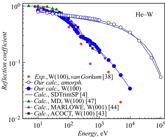
**Figure 7.** He–W system. Reflection coefficients for crystalline and amorphous target. ACOCT is an ACAT version for crystalline targets.
