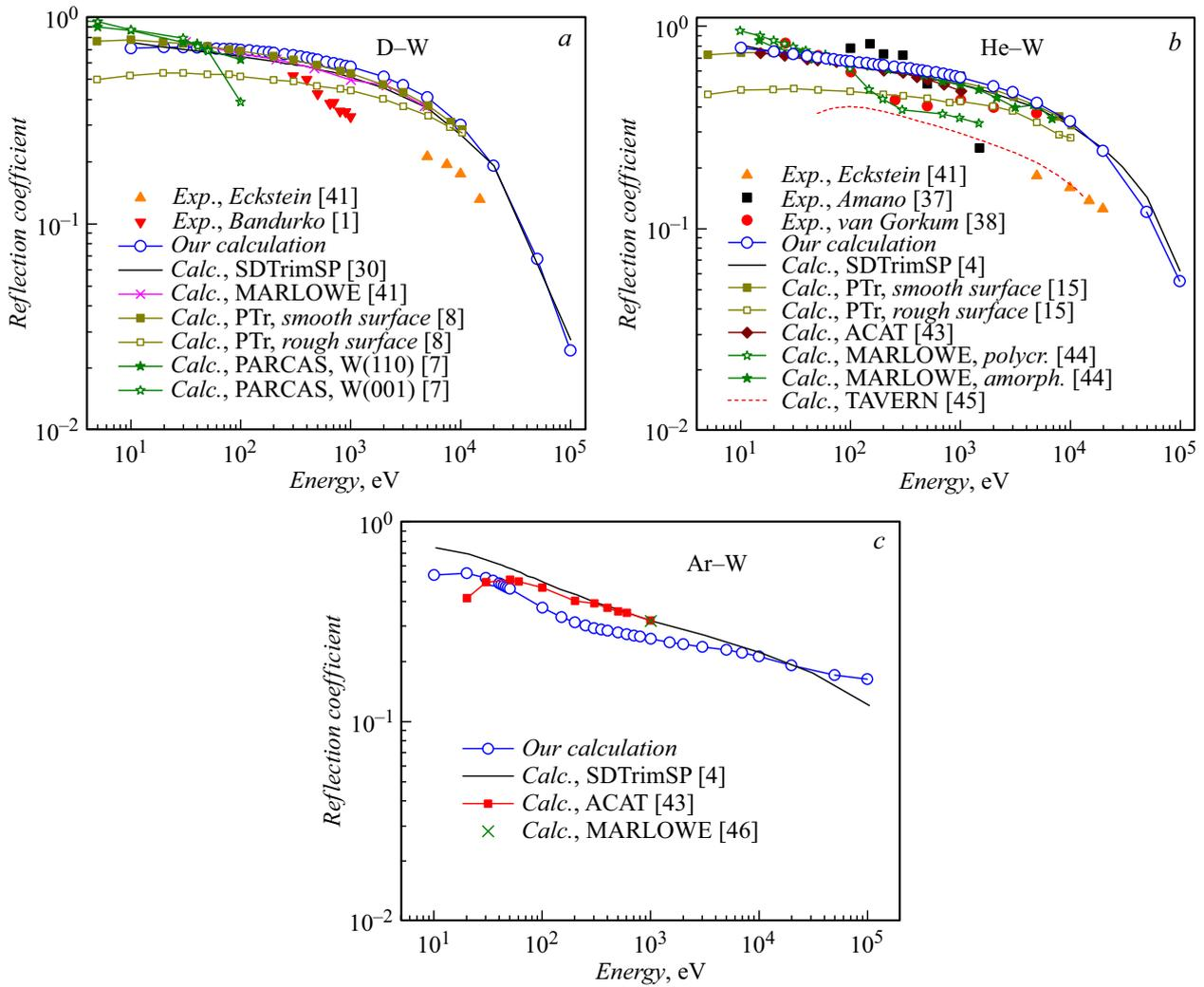
**Figure 6.** Reflection coefficients for D–W (a), He–W (b) and Ar–W (c) systems.
