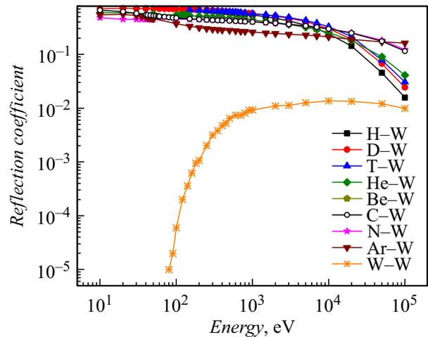
**Figure 2.** Calculated particle reflection coefficients for tungsten target depending on the energy for bombarding H, D, T, He, Be, C, N, Ar, W atoms. Data for W–W system is provided for the planar potential barrier.
