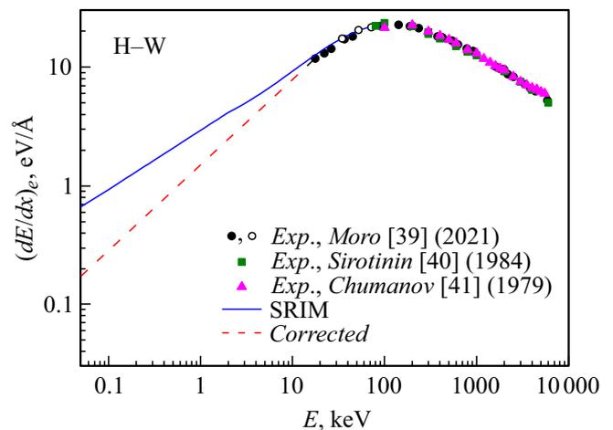
**Figure 5.** Dependence of electronic stopping on collision energy for H–W system. Dots — experimental data from [38–40]. Solid line — SRIM package data. Dashed line — modified data.
