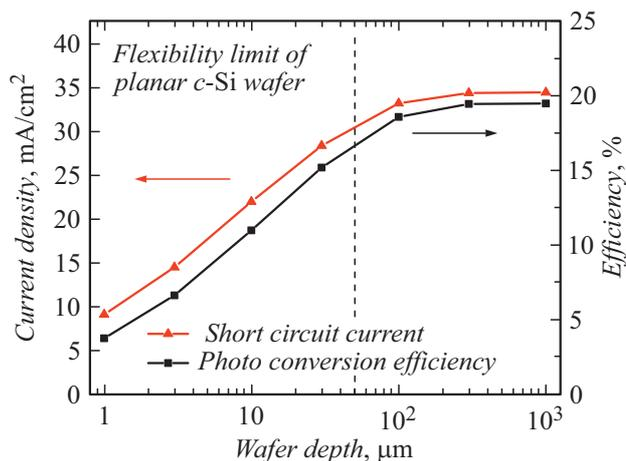
**Figure 3.** Calculated dependences of short-circuit current and solar cell efficiency on the silicon substrate thickness. The dashed line represents the flexibility limit of the silicon wafer.
