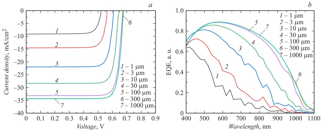
**Figure 2.** Calculated I-V curves under illumination with the AM1.5G spectrum (a) and external quantum efficiency spectra (b) for the PEDOT:PSS/Si heterostructures with different silicon substrate thicknesses.
