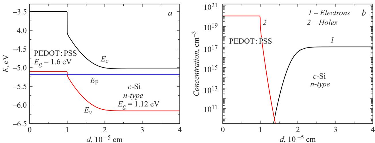
**Figure 1.** Calculated band diagram (*a*) and charge-carrier concentration distribution for the PEDOT:PSS/Si heterostructure (*b*).
